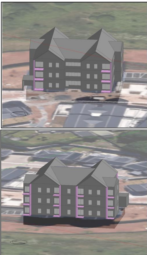
Figure 3 Example transient DesignBuilder model of the case study building
