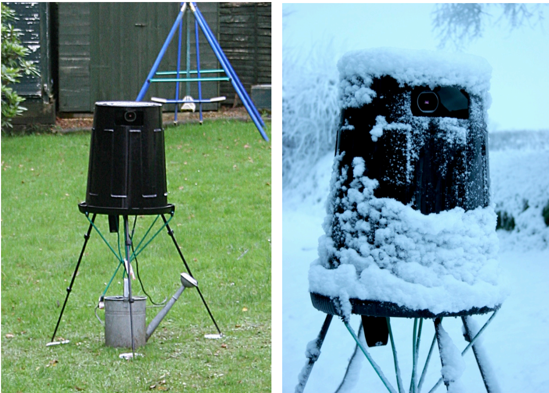
Figure 65. Tripod mounted thermal camera housed within a simple plastic shelter. (left). Snow covered experimental set-up (right).
