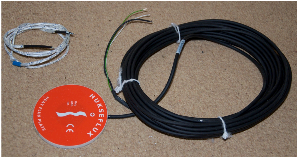
Figure 77. Hukseflux Heat flux sensor and K-type thermocouple.
