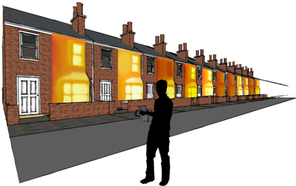
Figure 97. Illustration of walk-past thermography survey.
