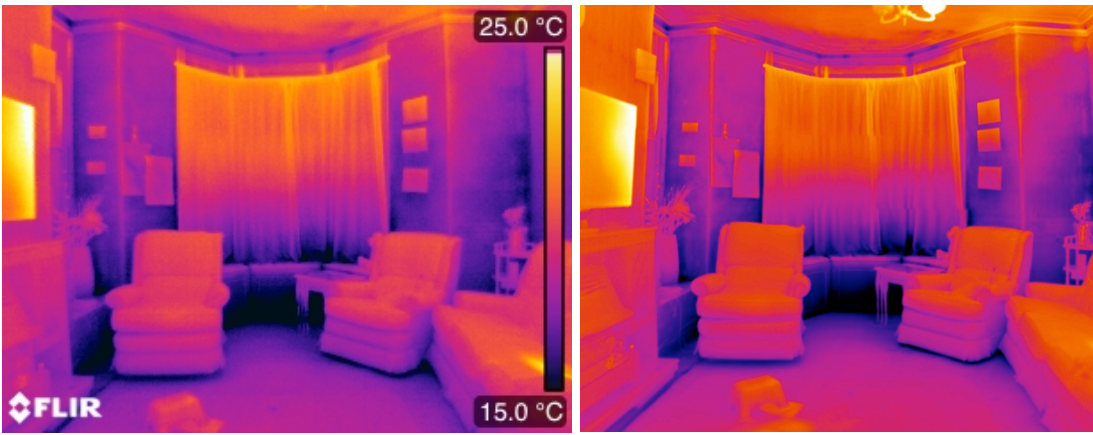
Figure 48. Single, wide-angle thermal image (Left). 16 individual thermal images pieced into one panoramic view (Right).
