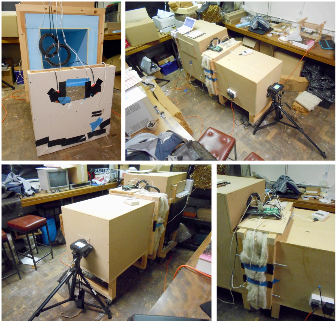
Figure 127. Four photos showing the sample, hot box, cold box and connected sensors.
