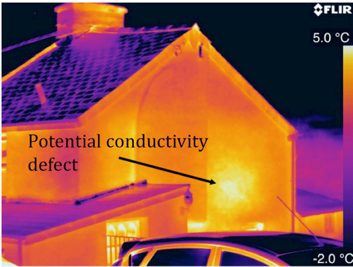
Figure 41. Potential conductivity heat loss through external wall.
