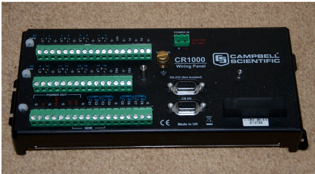
Figure 78. Campbell Scientific CR1000 data logger.
