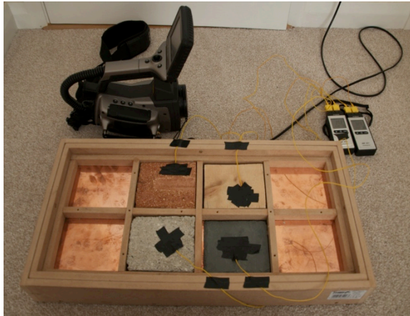
Figure 54. Photo of the experimental setup, thermocouples and IR camera.
