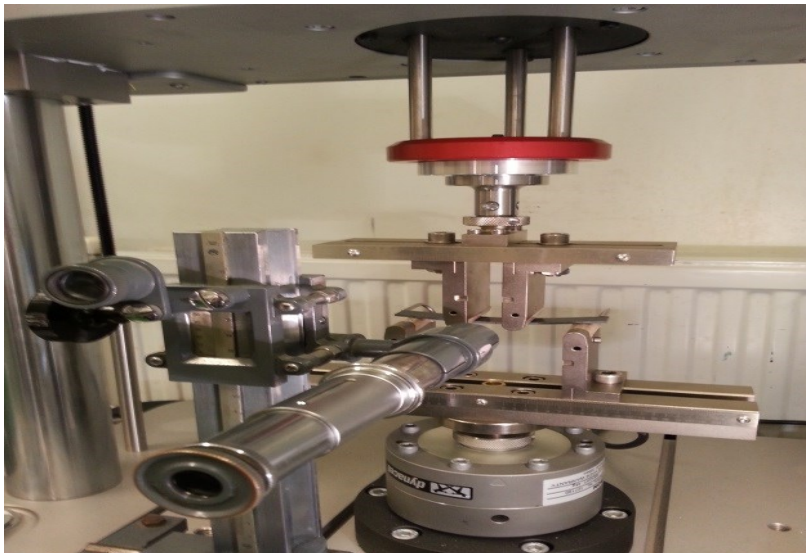
Figure B1-2: The travel microscope with the electro-pulse machine.
