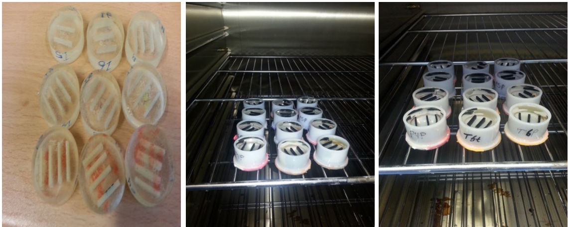
Figure B1-1: Casting the samples (from the infusion and RTM laminates) for image analysis.
