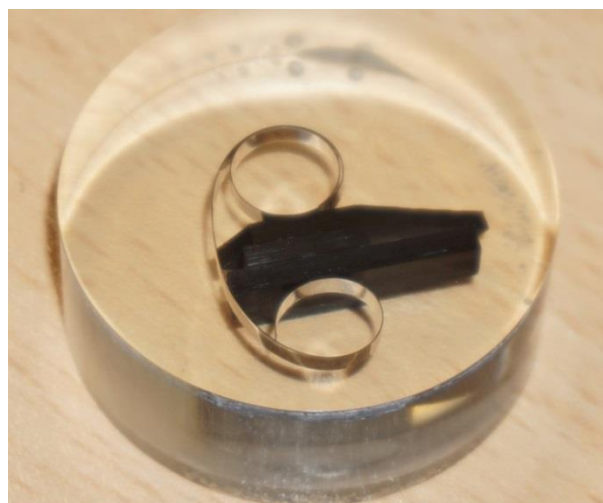
Fig.2 Polished UD ( [0]_{16} ), UT ( [90]_{16} ) and AP ( [\pm 45]_{4s} ) specimens for the microscopic study
