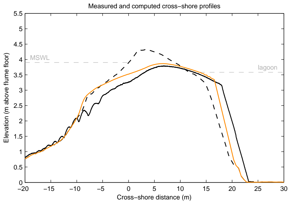
Figure 5.11: Initial cross-shore profile (---), cross-shore profiles measured (—) and modelled (—) at the end of wave series BAE10, and maximum still water levels (---).
