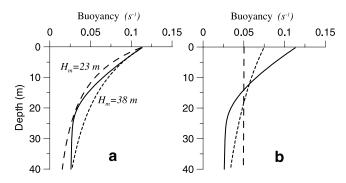
**Figure 14.** (a) The smoothed buoyancy frequency profile used in calculations (solid line) and two profiles defined by formula (2) for  $H_m = 23$  m (dashed line) and  $H_m = 38$  m (dotted line). (b) The buoyancy frequency profile used in Figure 16.
