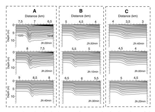
**Figure 11.** Density sections showing three stages of wave generation: frontal growth, wave fission, and free propagation for different values of density gradient: (a) large and sharp, (b) small and sharp, and (c) small and smoothed.
