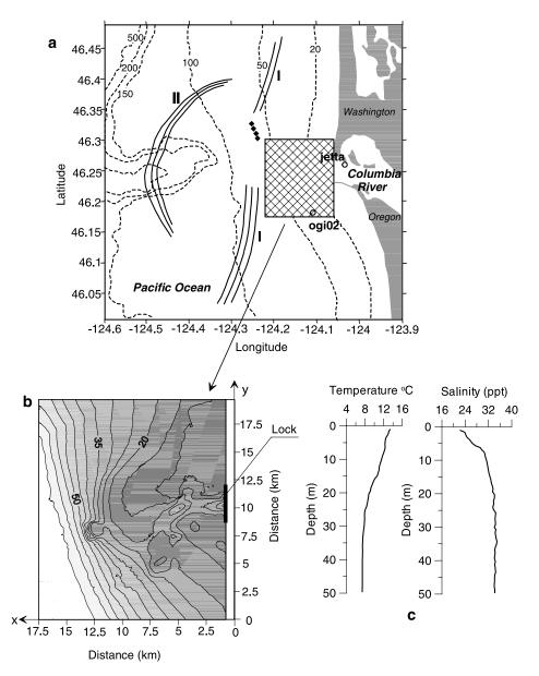
**Figure 1.** (a) The fragment of the Pacific Ocean showing the surface manifestations of IWs (marked as I and II) acquired by SAR. The black diamonds spot the position of measurements [*Nash and Moum*, 2005]. Two open circles show the location of CTD stations: "Jetta" and OGI02. The shaded rectangle designates the model domain. (b) Zoom of the model domain. (c) The profiles of the background temperature and salinity on the shelf.
