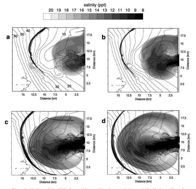
**Figure 9.** Surface salinity field after t = 6 hours of the plume evolution overlaid with the gradient of horizontal velocity and bottom topography: (a) motion is initiated by the density difference between estuary and ocean; (b) the density gradient is accompanied by the river discharge; (c) the density gradient is accompanied by the tide; and (d) the density gradient, tide, and river discharge act together.
