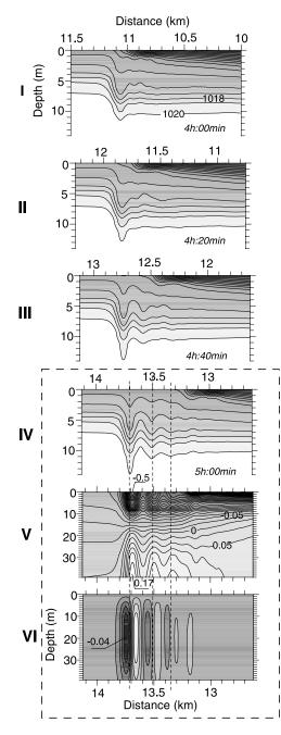
**Figure 6.** Density sections showing three stages of wave generation: (I) frontal growth, (II) wave fission, and (III) free wave propagation. Dashed rectangle: (IV) additional density section with corresponded (V) horizontal and (VI) vertical velocities (contour labels in m s<sup>-1</sup>).
