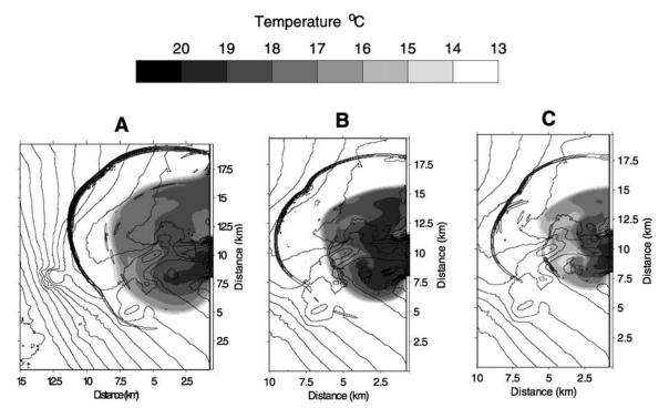
**Figure 10.** Surface temperature at t = 5 hours overlaid with the gradient of horizontal velocity  $G > 10^{-3}s^{-1}$  and bottom topography for different values of density gradient: (a) large and sharp, (b) small and sharp, and (c) small and smoothed (see explanation in text).
