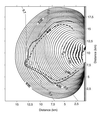
**Figure 7.** The position of the plume boundary presented with a 10-min interval (black thin and thick lines). Two thick gray lines show the contours of the linear phase speed in m s<sup>-1</sup>. The thick dashed line shows the locations of the actual wave separation from the plume. The dotted curve indicates the positions of Fr = 1 calculated from linear boundary value problem (1).
