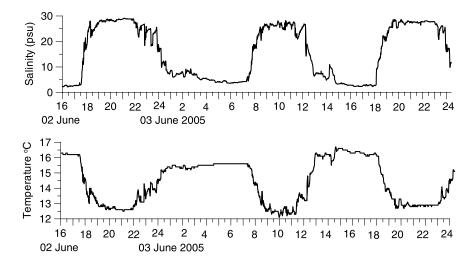
Figure 2. Example of CTD measurements in the river mouth at depth of 6.4 m (station Jetta).
