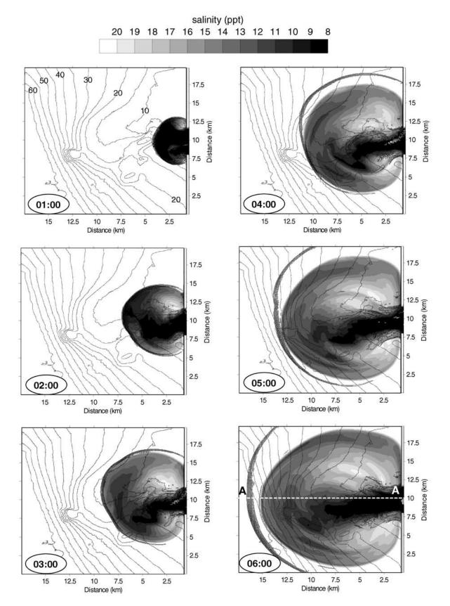
Figure 4. Time series presenting the surface salinity (gray for fresh water and white for saline water) overlaid with the maximum gradient of horizontal velocity ( $G > 10^{-3} \text{ s}^{-1}$ , black lines) and bottom topography.
