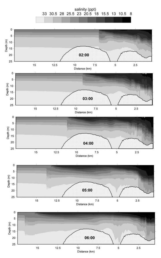
Figure 5. Evolution of the salinity field in the cross section A-A (see Figure 4).
