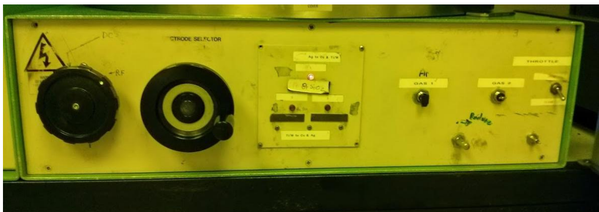
Figure 4 – The target or ‘electrode selector’ is the second wheel to the left. The lights on the panel to the right indicate which target is selected. The first switch on the right turns the argon supply on and off. The knob immediately down and to the right controls the argon pressure. The toggle switch on the far right is the throttle
