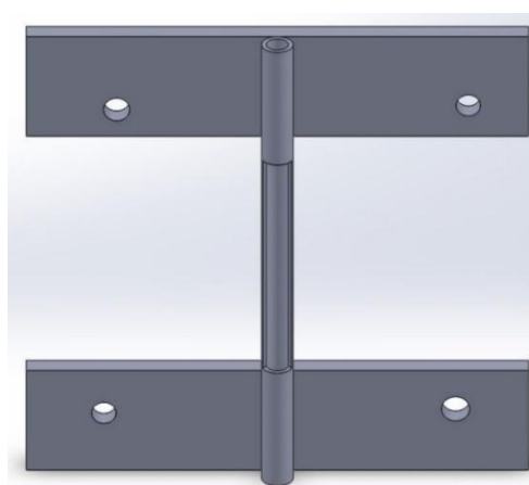
Figure 4.10: The 4-spring based tightening mechanism used to secure the prism, thin-layered system and the micro-fluid channel, 3D design of the base of the mechanism.
