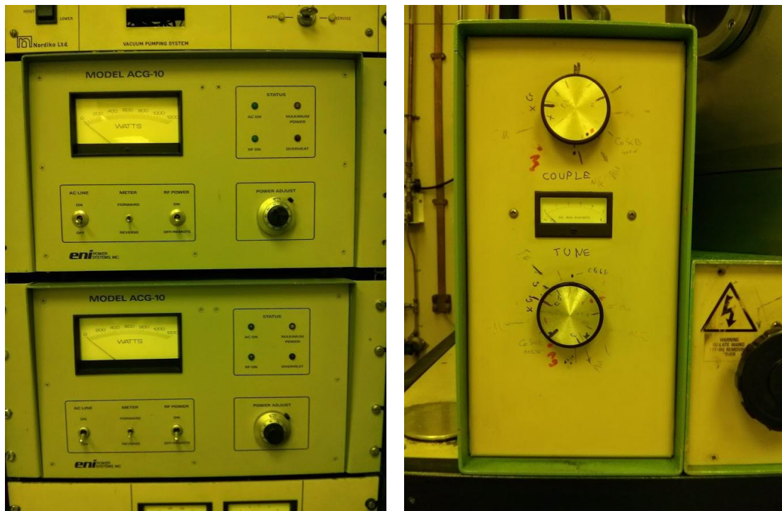
Figures 2 and 3 – The two power supplies are on the left. The top is for the substrate and the bottom is for the target. On the right are the tuning and coupling dials. Note the markings for rough positioning
