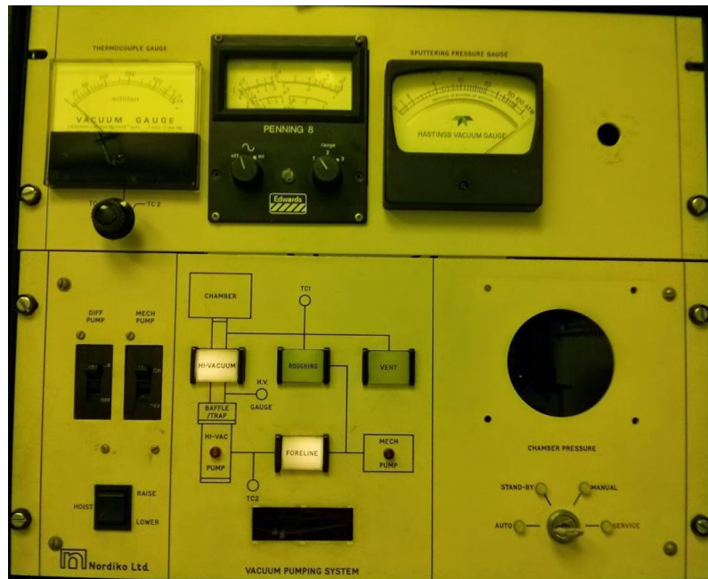
Figure 1 – The mechanical and diffusion pump switches are on the bottom left. The buttons for hi-vac, roughing, vent and foreline are in the bottom centre. The middle and right hand pressure dials are at the top
