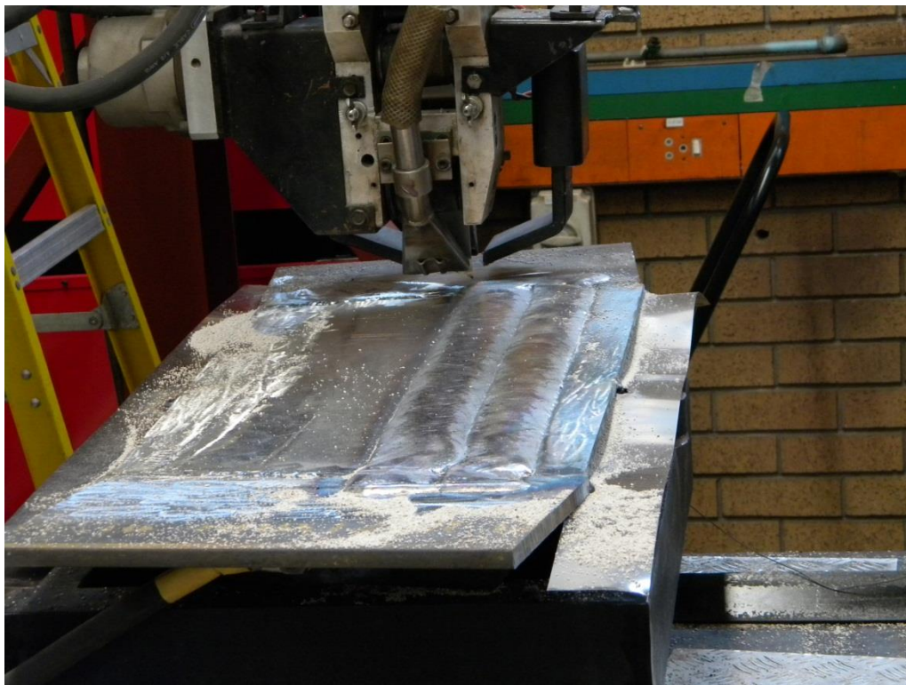
Figure 2 View of the coupon after laying down two weld runs. The four edging tabs can be clearly seen in the image.
