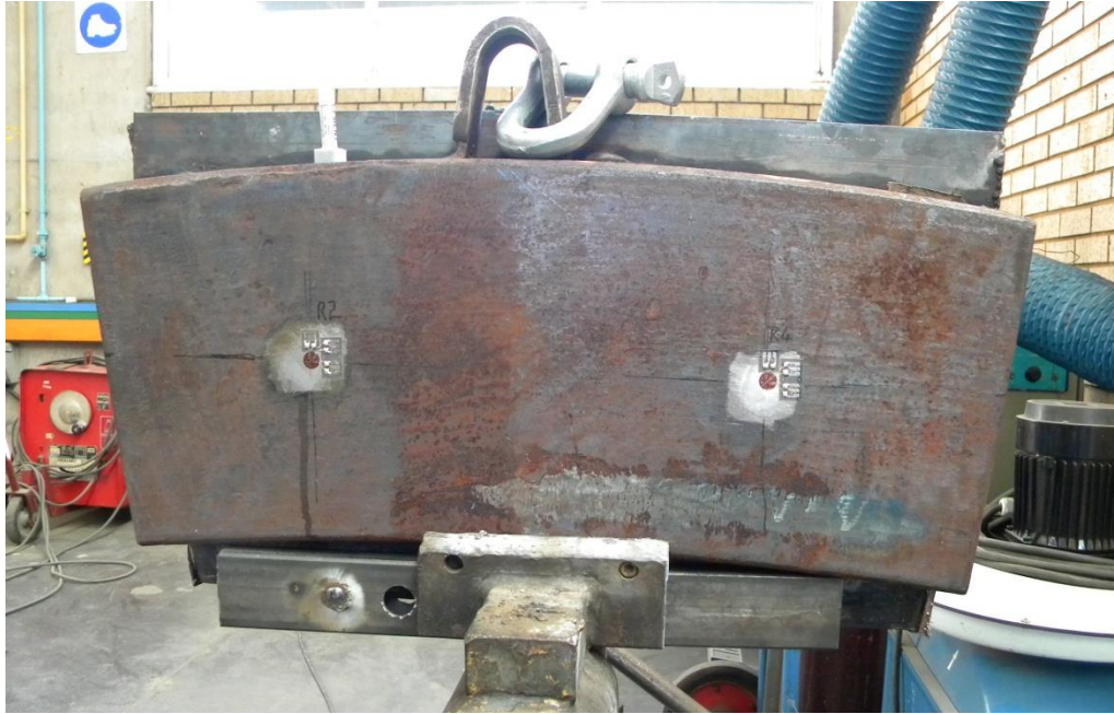
Figure 1 View of the A533B Class 2 steel coupon from the side opposite the cladding. The image shows the curved shape of the original RPV wall. It should be noted that in actual reactor use the cladding would be applied to the inner curved face.
