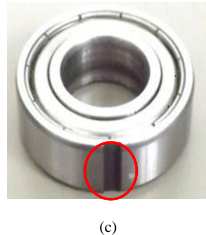
Figure 4.8 Outer race rack fault with different severities: (a) 0.2x1x3 mm, (b) 0.5x1x6 mm and (c) 3x1x9 mm
