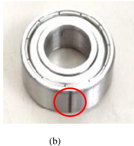
Figure 4.8 Outer race rack fault with different severities: (a) 0.2x1x3 mm, (b) 0.5x1x6 mm and (c) 3x1x9 mm
