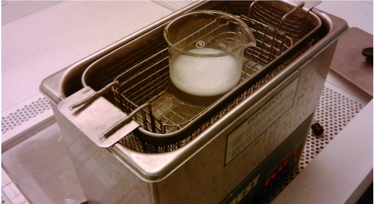
Figure B.1 bearing cleaning and remove lubrication for experimental test
