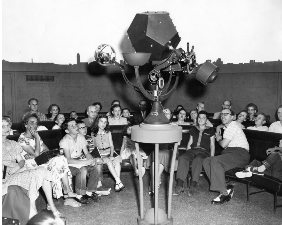
Figure 54. Spitz Model A1 planetarium projector (1955).
