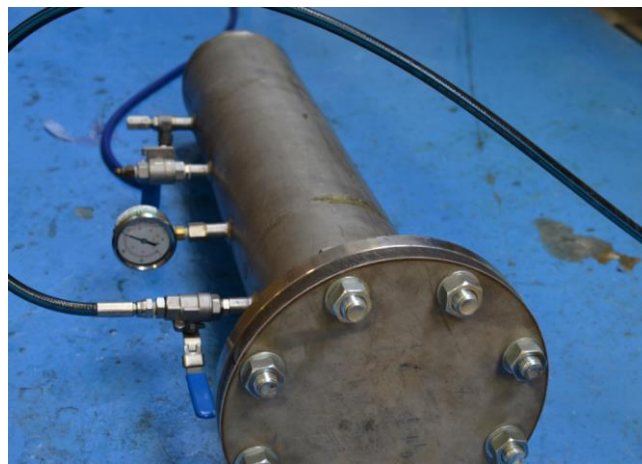
Fig.3. The hydrostatic chamber used in the diffusion test.
