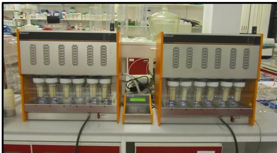
Figure 5.4: Soxhlet system operated in the nutrition laboratory of the University of Plymouth.
