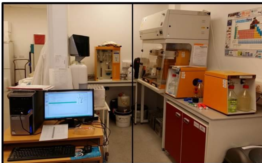
Figure 5.5: Left is computerized digestion block and right is distillation unit of the Kjeldahl system utilized (Gerhardt Laboratory instruments) at the University of Plymouth.
