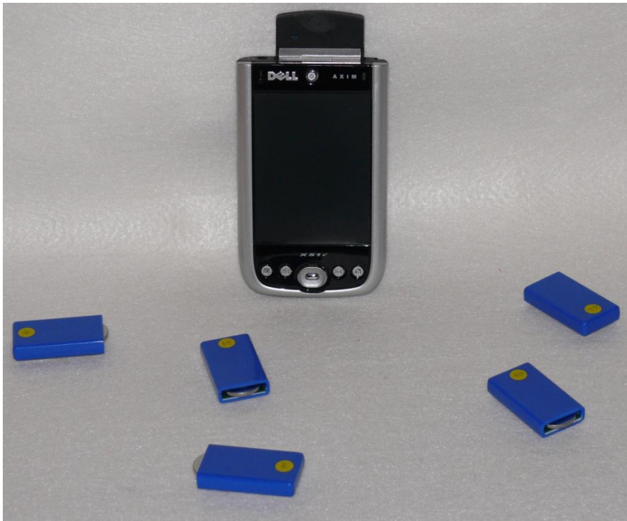
Figure 4-2. A PDA with installed RFID node and five RFID tags
