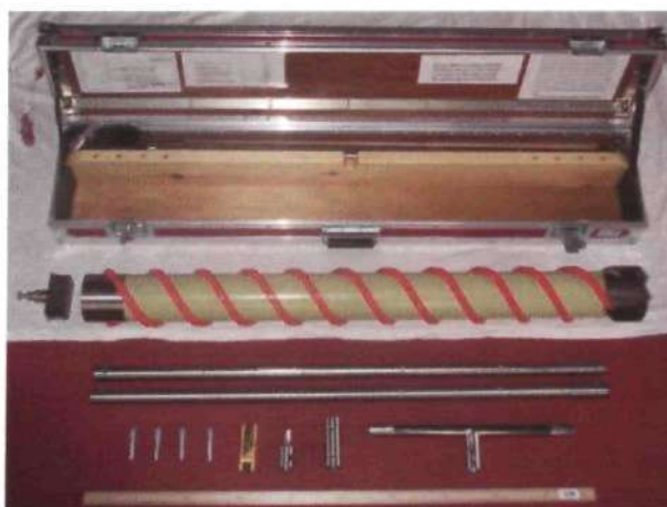
Figure 4.3-3. Kovacs Enterprises © Mark II sea ice corer and accessories used to collect sea ice samples during the IPY-CFL cruise, 2008 (Kovacs, 2010).
