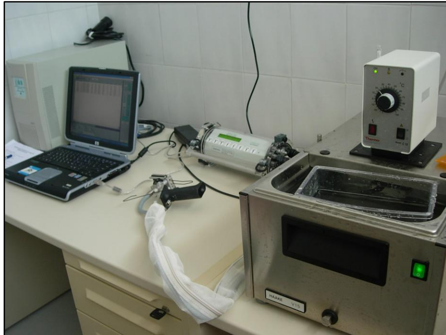
Figure 22. Laboratory set up of the PAM fluorometer and the Haake open cryostat circulator for measuring photosynthetic activity of Cymodocea nodosa shoots.
