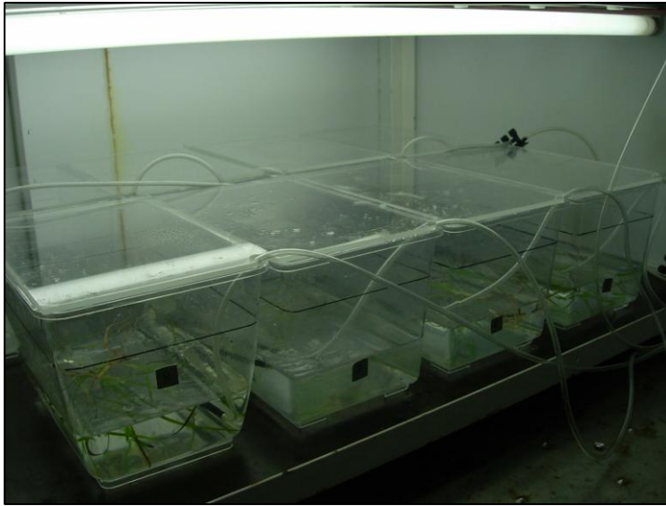
Figure 37. Experimental set up of plastic containers with Cymodocea nodosa shoots, oxygenated and kept in a controlled temperature room.
