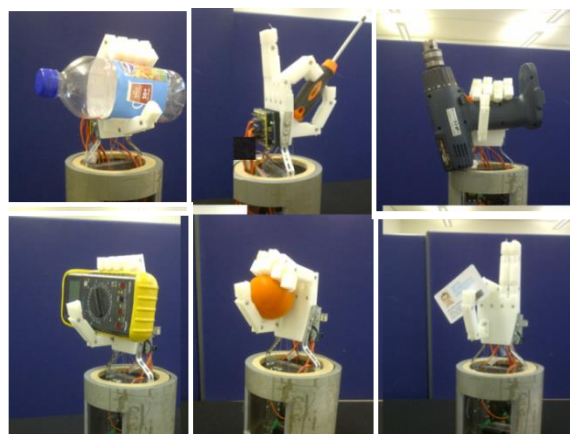
Figure 5.21 Examples of grasping different light and heavy objects with the dextrous robotic hand (Brochard, 2012). Permission to reproduce this figure has been granted by Alex Brochard
