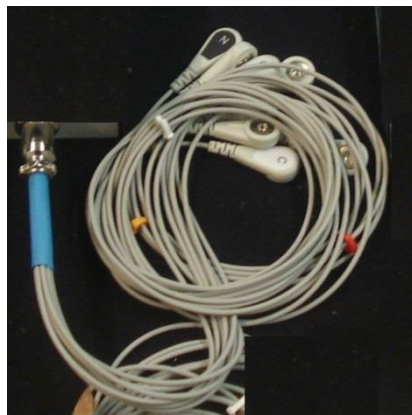
Figure 5.7 The EMG lead wires with press stud for 4 EMG channels
