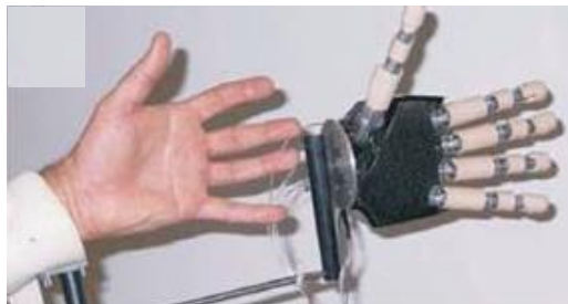
Figure 3-34 The CyberHand with the externally actuated motor (Carrozza et al., 2006). Permission to reproduce this figure has been granted by Springer.
