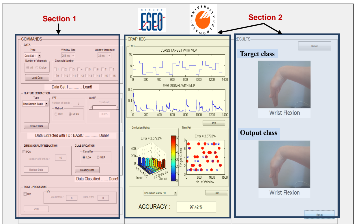
Figure 5.13 The GUI of the offline PR system. The selection of pattern recognition techniques is shown on the left side (shown in red). The visualization section of the classification output is shown on the middle and right parts of the GUI (shown in yellow and blue)
