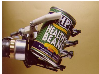
Figure 3-21 Power grip with the Southampton hand (Light and chapel 2000). Reprinted from Medical Engineering & Physics, 22(10), C.M. Light and P.H. Chappell, Development of a lightweight and adaptable multiple-axis hand prosthesis, pp 679-684, Copyright (2000), with permission from Elsevier.
