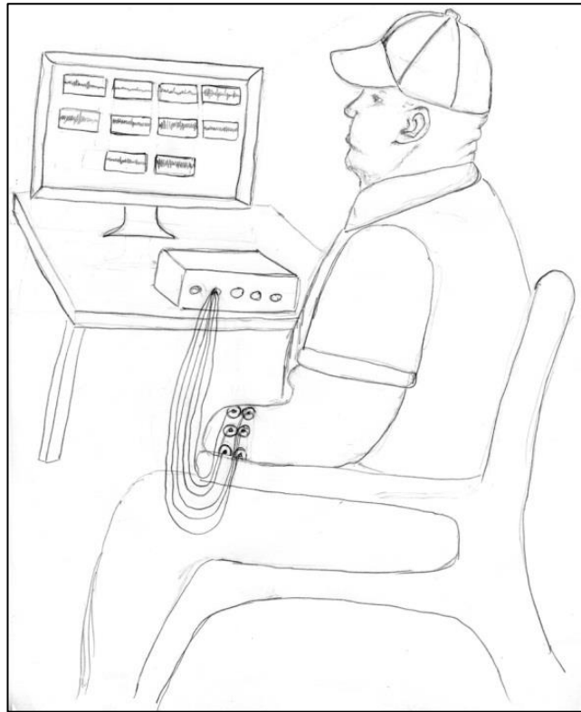
Figure 9.3 An illustration showing the experimental setup with an amputee using the visual feedback from the EMG signals to perform the required movement.
