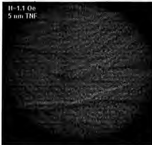
(b) Showing domain walls at H_a = 1.1 Oe or 84 A/m
