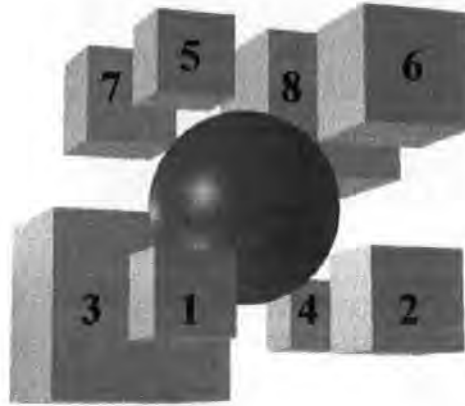
Figure 8.3 Calculation of the hard sphere diameter, D_h .
