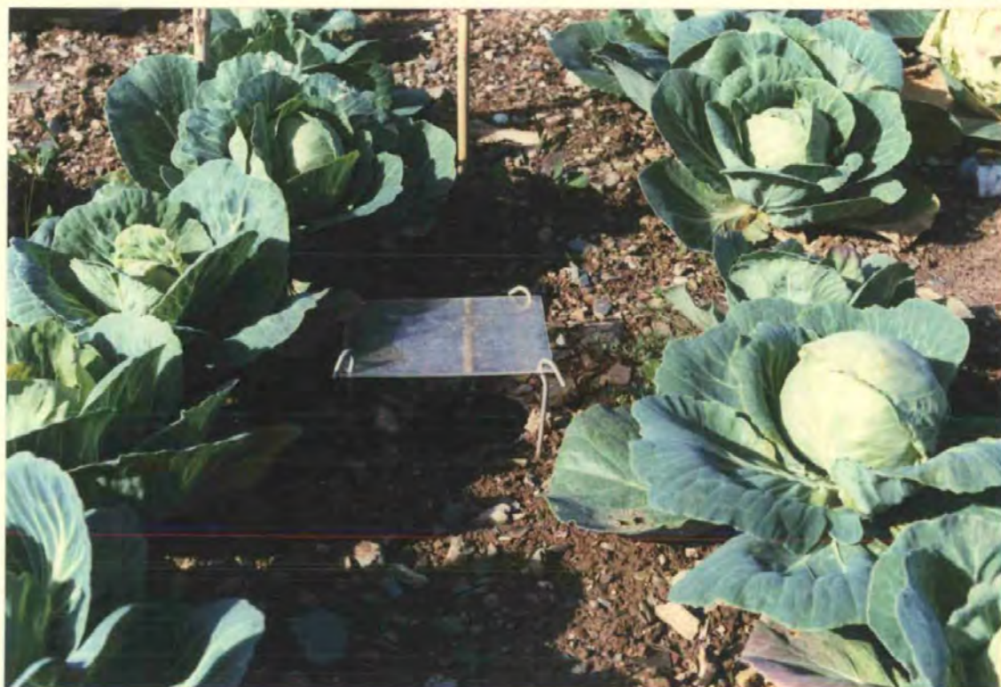
Figure 2.2b: Pitfall with protective roof
