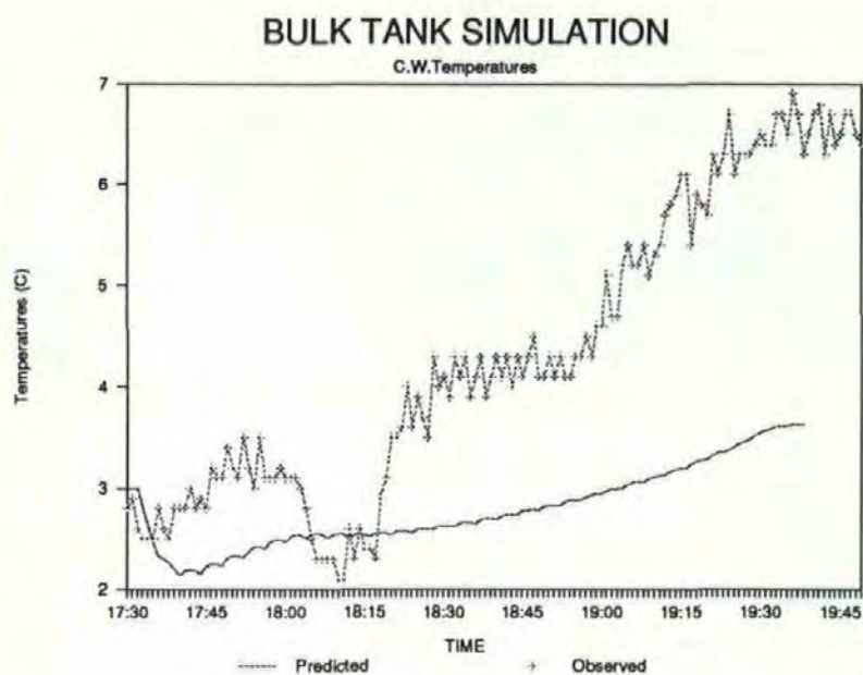
Figure 4.3 (b) Observed and predicted chilled water temperatures from the laboratory simulation.
