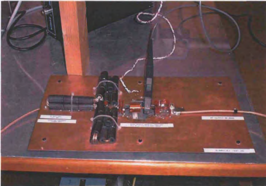
Figure 3.6 – Current Transformer used in High Power Measurements
