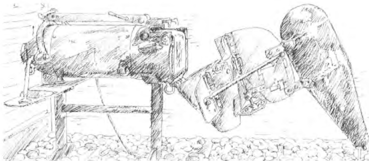
Figure 2.6. Original Hardy Continuous Plankton Recorder, 1925 (source: Andy Bleck).
