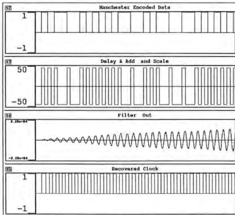
**Figure 2-15 Acquisition performance - Manchester encoded data**
