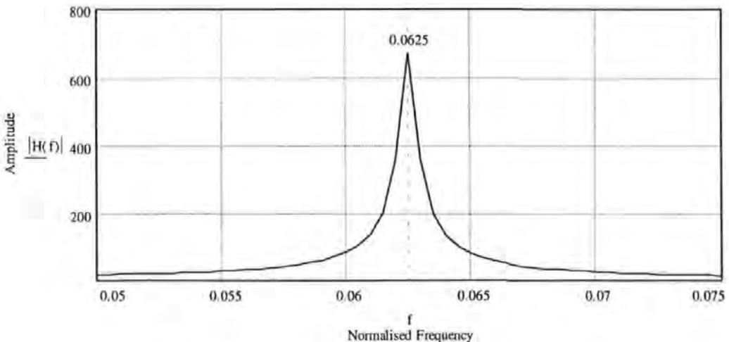
**Figure 2-10 Frequency response of the IIR filter**
