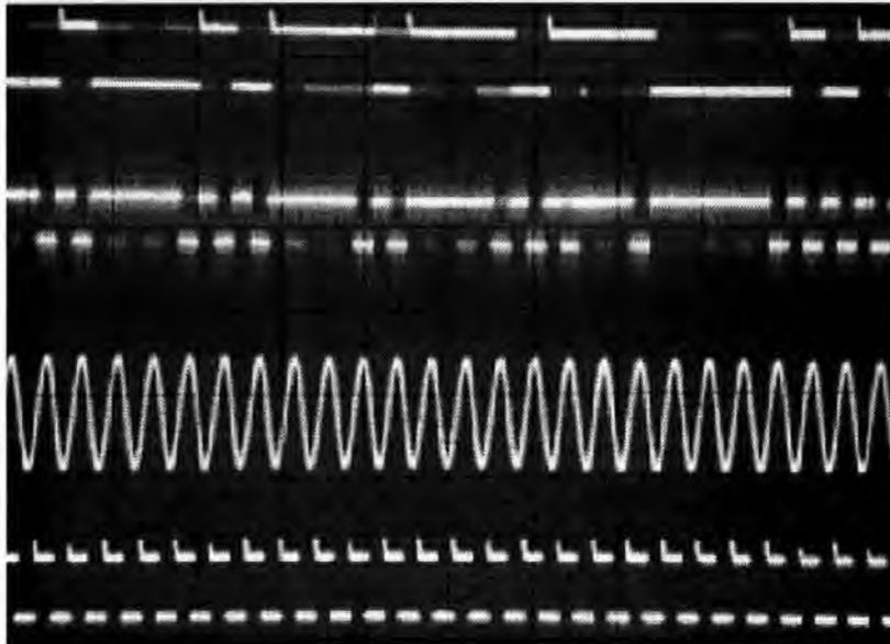
**Figure 2-31 Oscilloscope display of clock recovery signals**
