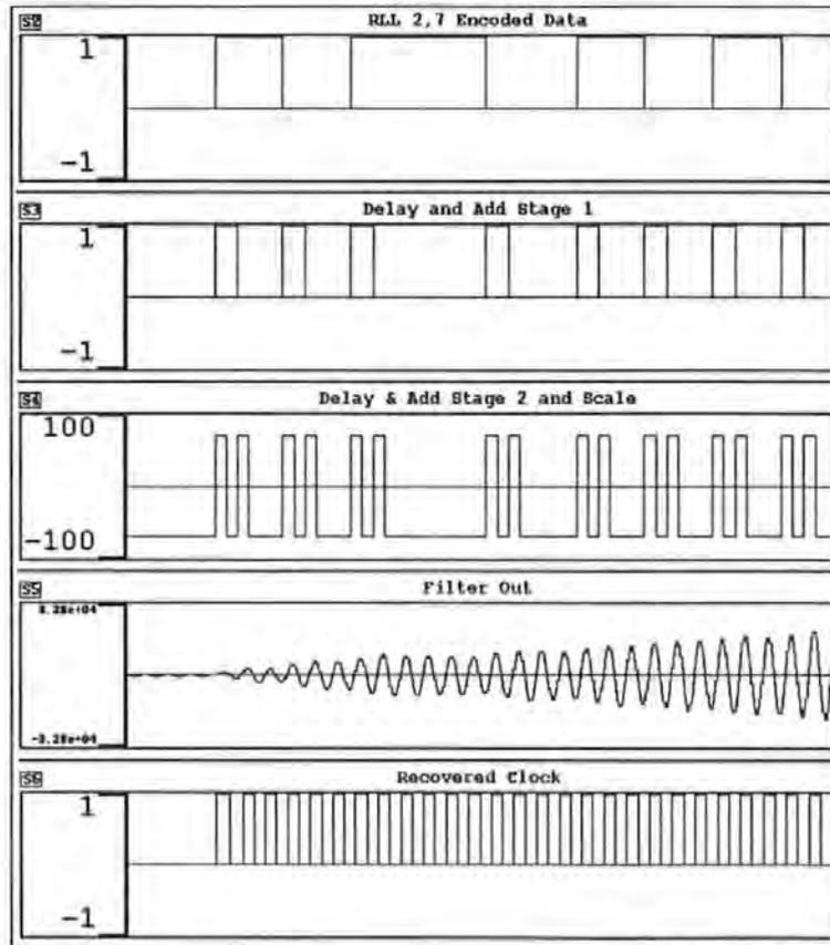
**Figure 2-16 Acquisition performance - RLL 2,7 encoded data**
