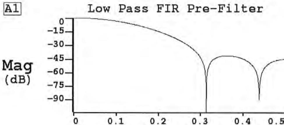
**Figure 3-21 Pre-filter frequency response**
