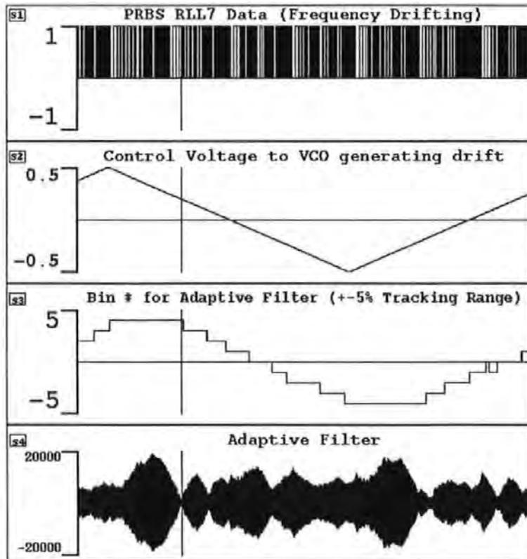
Figure 3-40 Tracking performance  $\pm 5\%$  range - RLL7 data
