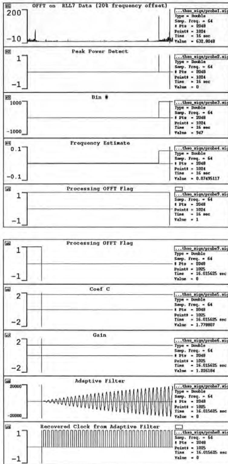
Figure 4-10 Simulation of clock recovery using OFFT
