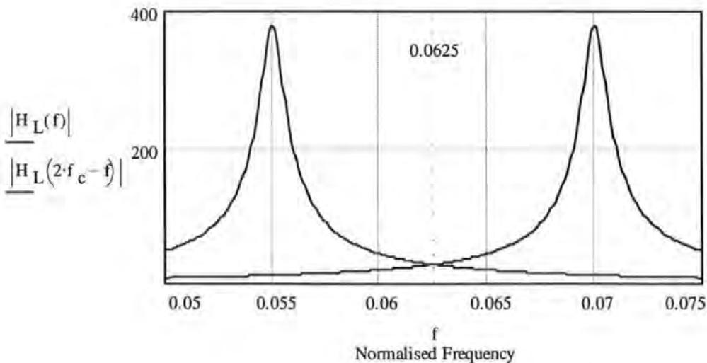
**Figure 3-6 Ideal mirrored detection filters**
