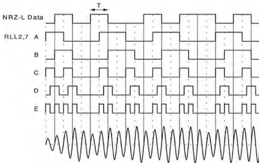
**Figure 2-8 Timing diagram for 1/2 rate codes**
