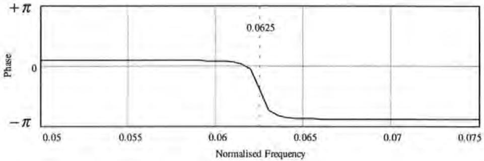
**Figure 2-11 Phase response of the IIR filter**
