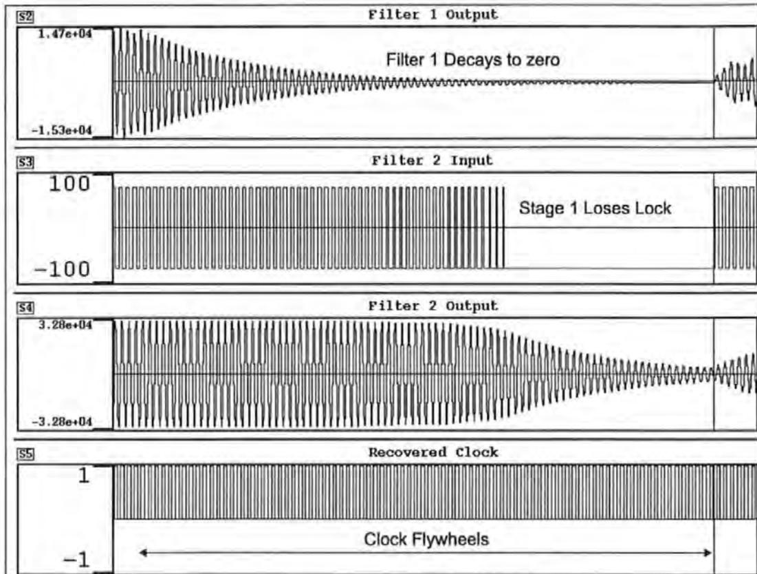
Figure 2-21 Flywheel performance - Two stage filter (NRZ data)
