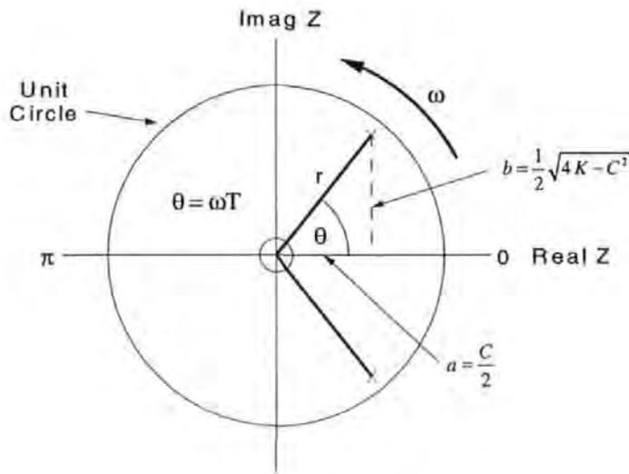
Figure 2-12 Z-Plane diagram
