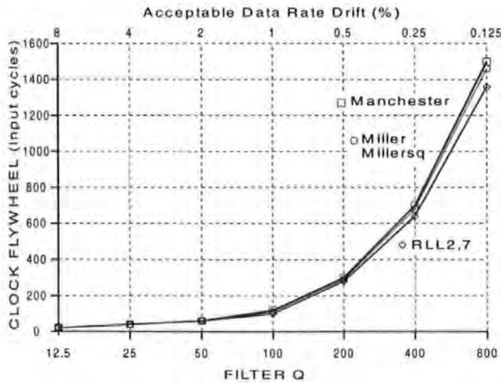
**Figure 2-17 Filter-Q versus flywheel**
