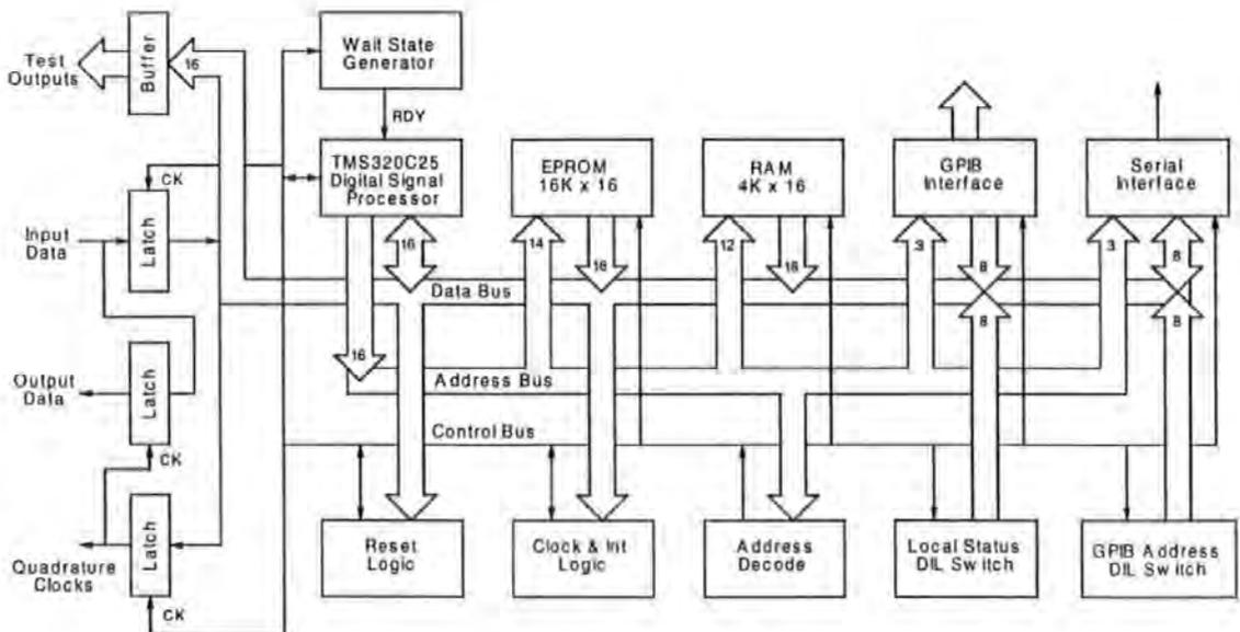
Figure 2-27 DSP-based clock recovery hardware - Block diagram
