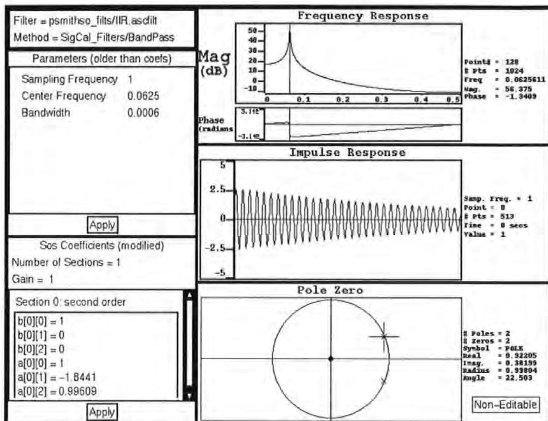
Figure 2-13 Filter design analysis
