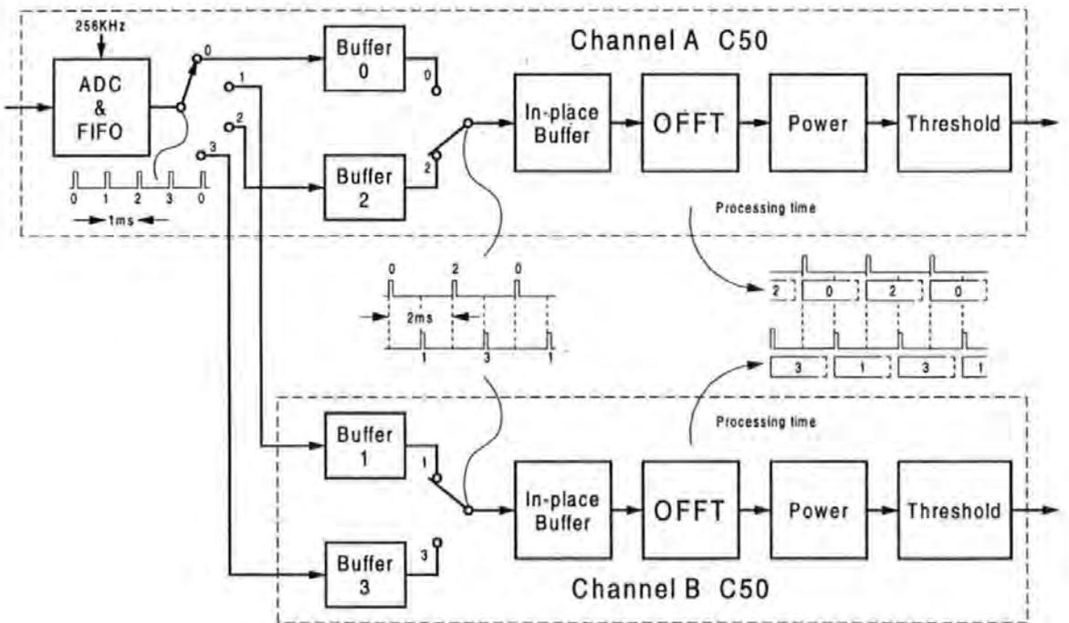
**Figure 4-13 OFFT implementation using flip-flop dual buffers**
