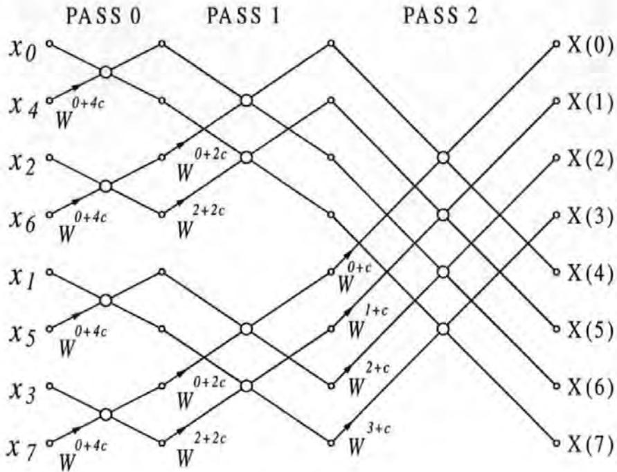
Figure 4-14 Flow diagram for an 8-point OFFT
