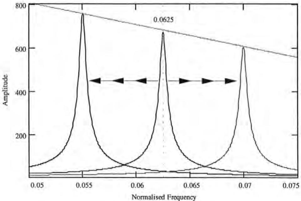
**Figure 3-3 Tracking filter with no amplitude compensation**
