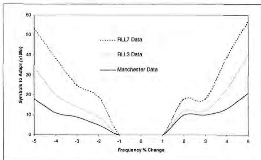
Figure 3-29 Acquisition performance -  $\pm 5\%$  tracking range
