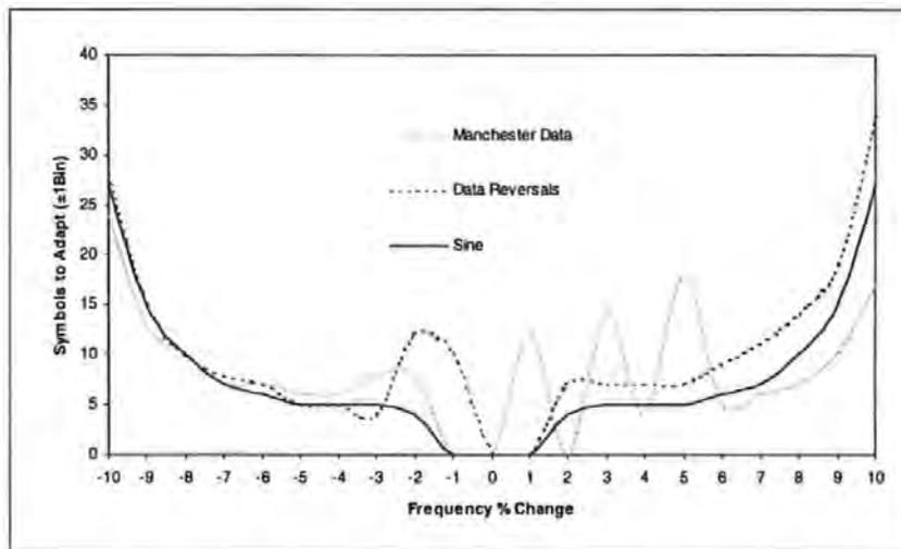
**Figure 3-32 Acquisition performance -  $\pm 10\%$  tracking range**
