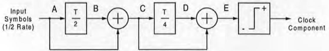
**Figure 2-7 Two stage Delay and Add conditioner**
