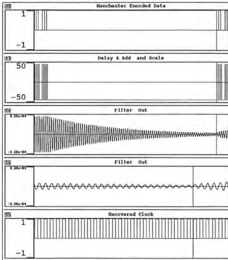
**Figure 2-18 Flywheel performance - Manchester encoded data**
