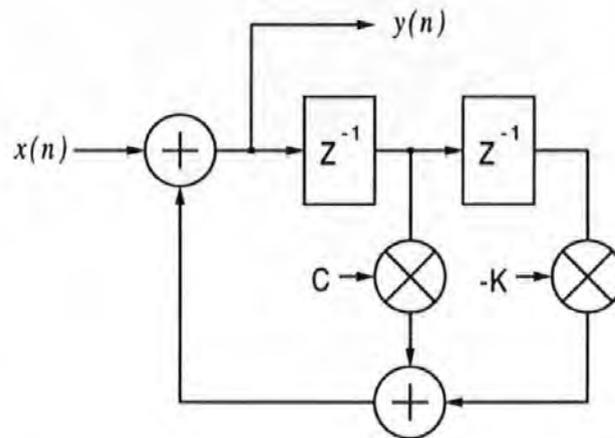
Figure 2-9 Architecture of clock recovery IIR filter
