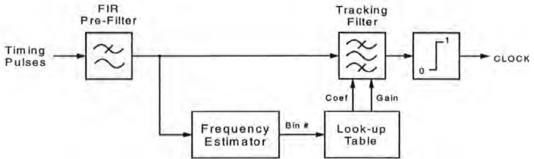
**Figure 3-20 Adaptive filter for use with rectangular pulses**
