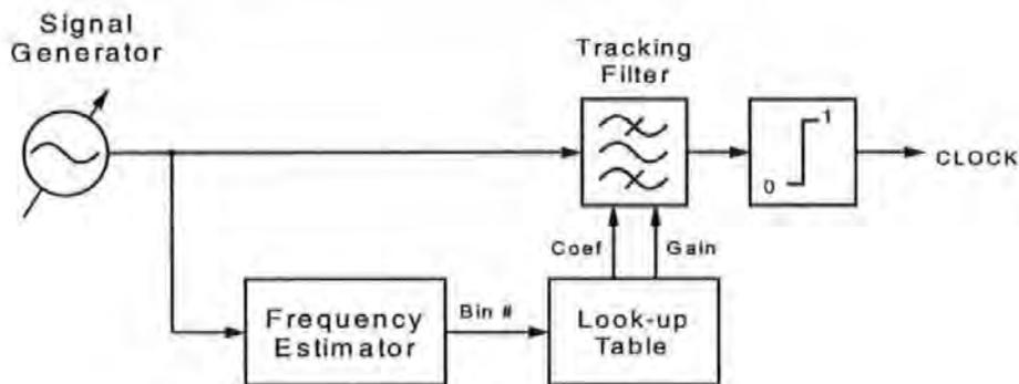
**Figure 3-15 Overview of adaptive filter test model**
