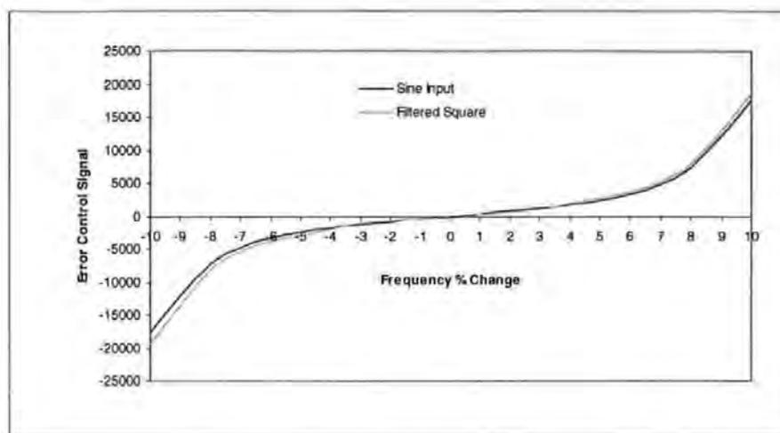
**Figure 3-22 Error control signal with a pre-filter**
