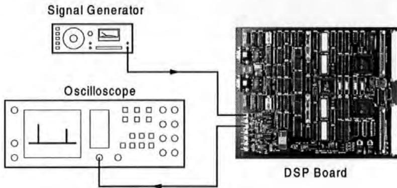
**Figure 4-15 The OFFT test arrangement**
