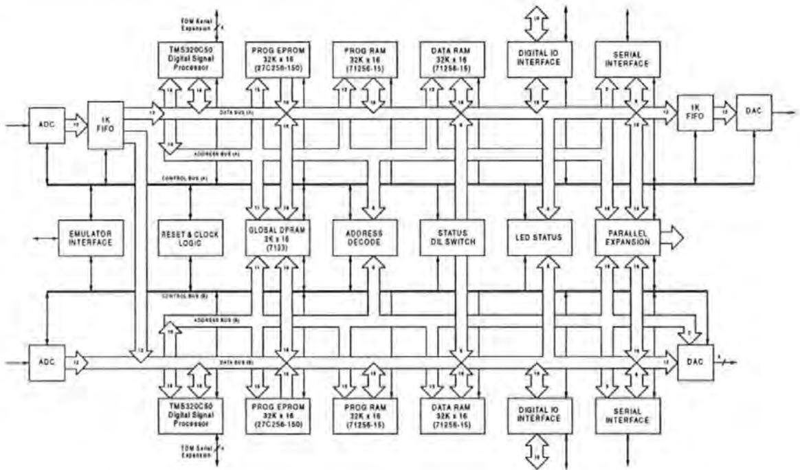
**Figure 4.11 Dual-processor DSP hardware - Block diagram**
