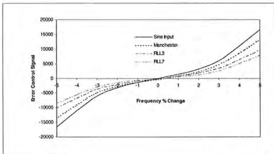
Figure 3-26 Error control signal for  $\pm 5\%$  offset
