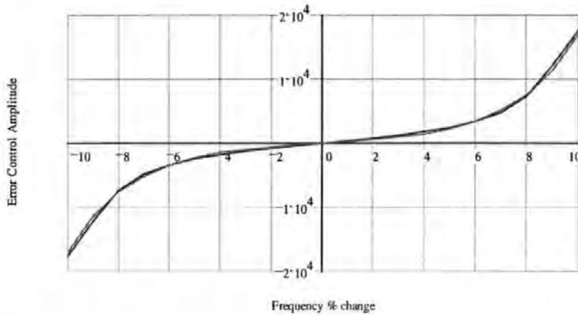
**Figure 3-11 Error calibration over ±10% frequency offset**
