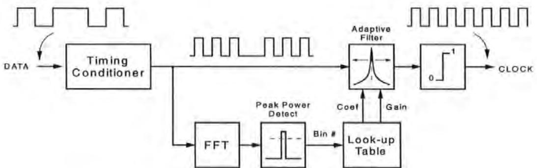
Figure 4-1 Concept of FFT-based adaptive clock recovery
