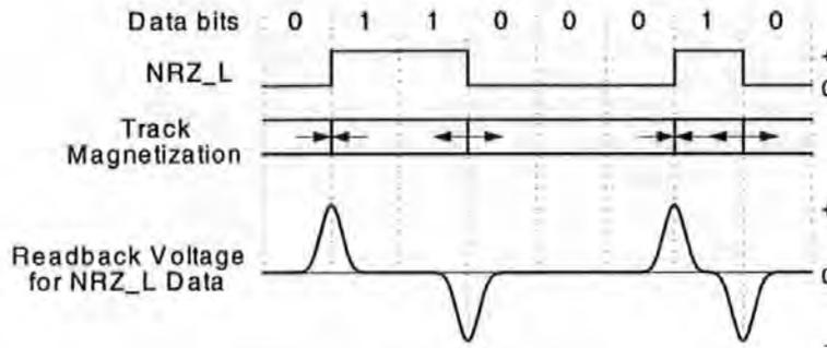
**Figure 1-17 Saturated magnetic recording**
