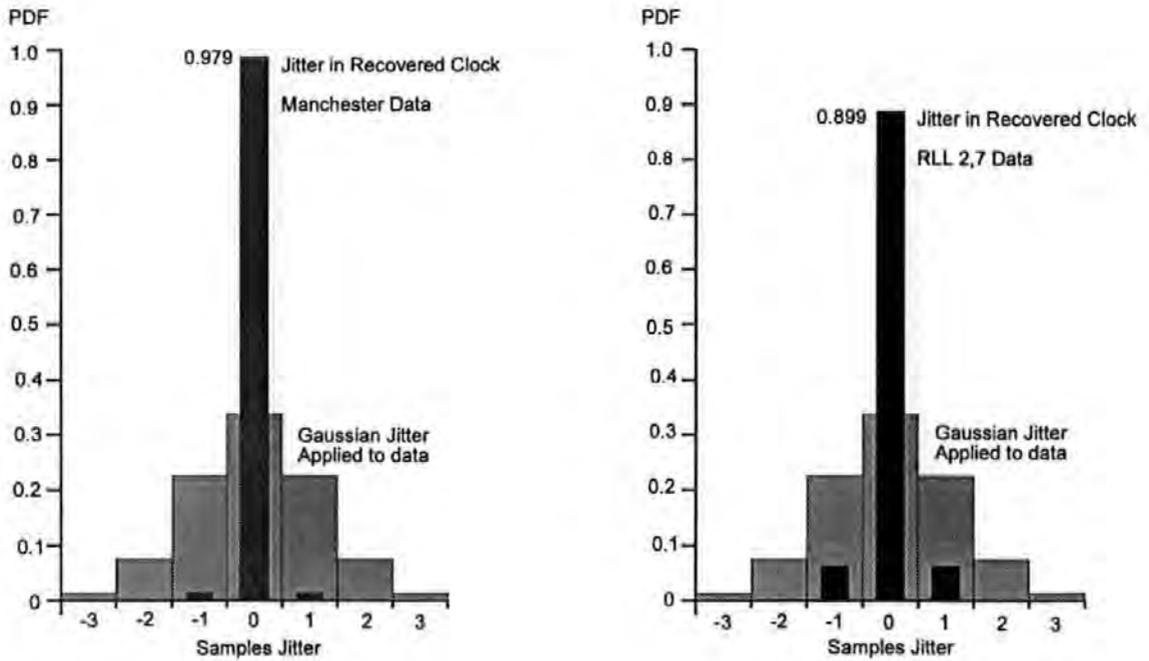
Figure 2-25 PDF of jitter in the recovered clock
