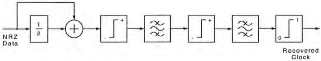
Figure 2-20 Two-stage filter section
