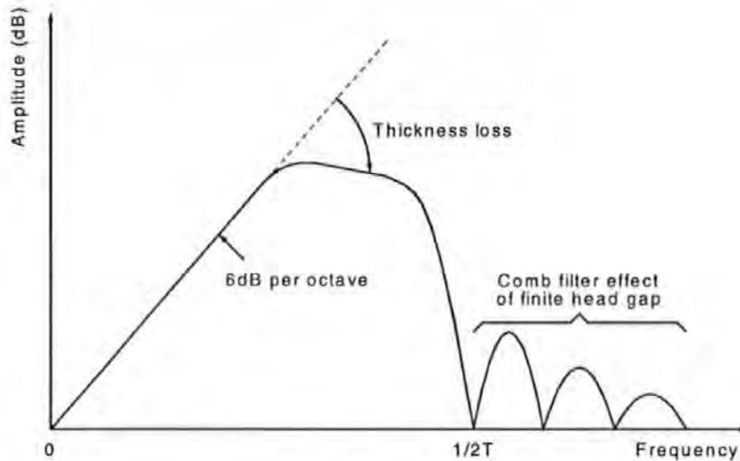
**Figure 1-15** Frequency response of a recording channel
