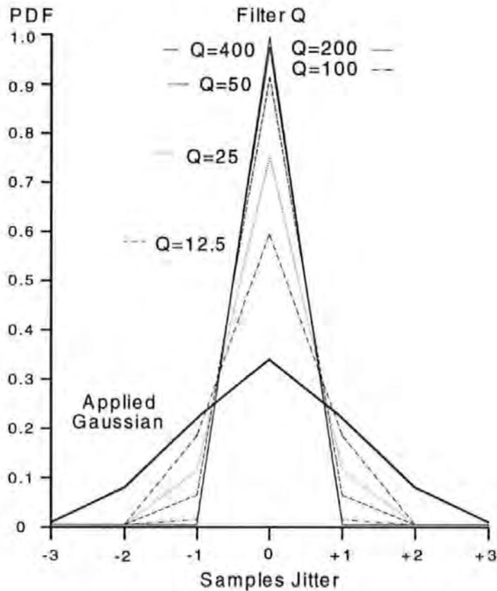
Figure 2-26 PDF of jitter versus Filter Q - Manchester data
