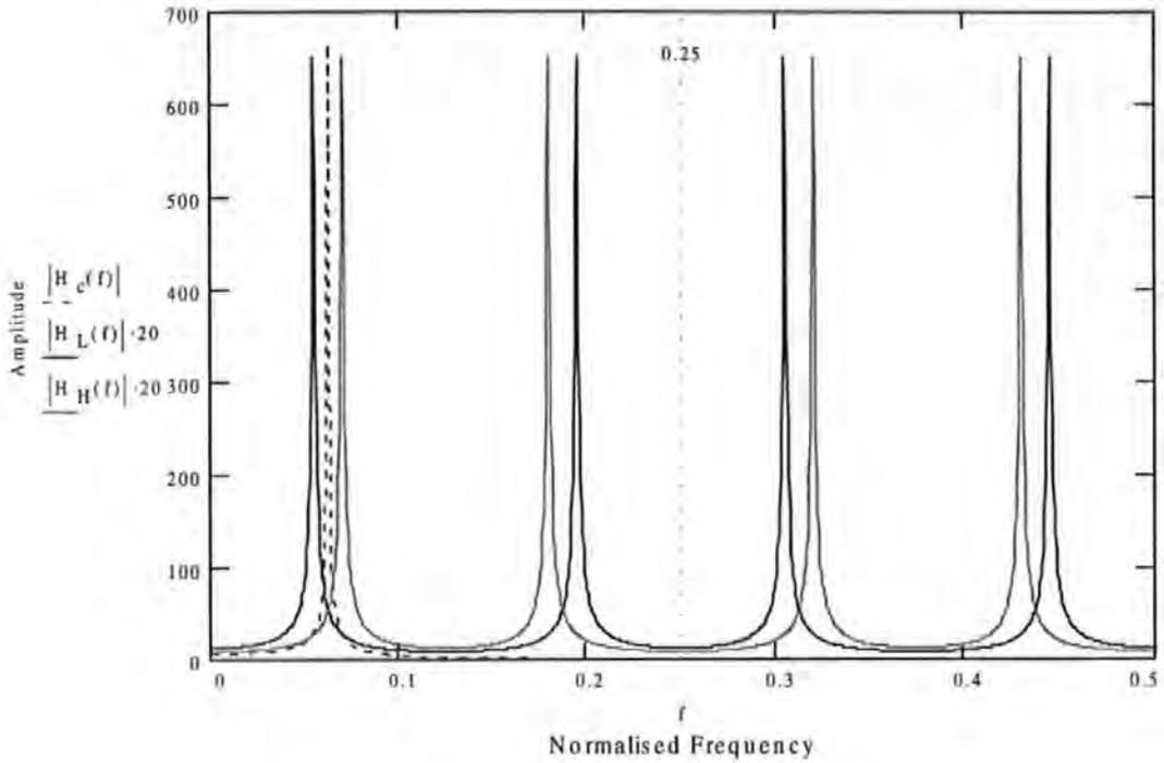
**Figure 3-9 Repeat spectrum of detection filters**
