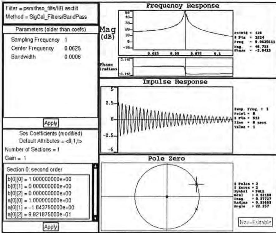
Figure 2-35 IIR Filter quantized to 9 bits
