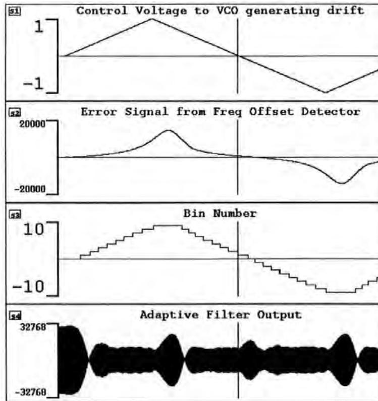
**Figure 3-38 Tracking performance  $\pm 10\%$  range - Sine input**
