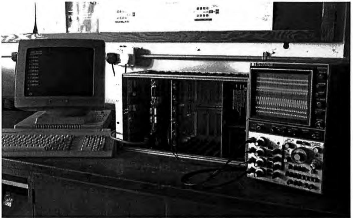
**Figure 2-30 Clock recovery test system**
