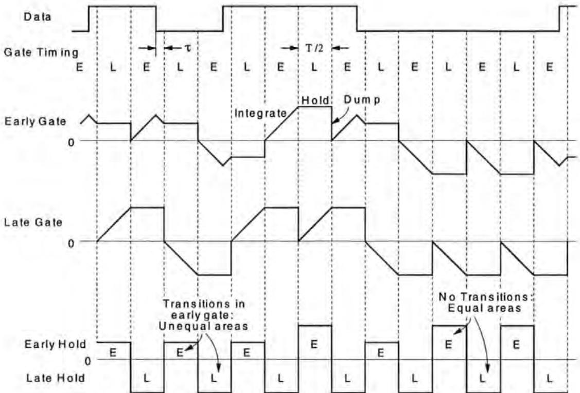
Figure 1-12 Timing diagram for early-late synchroniser
