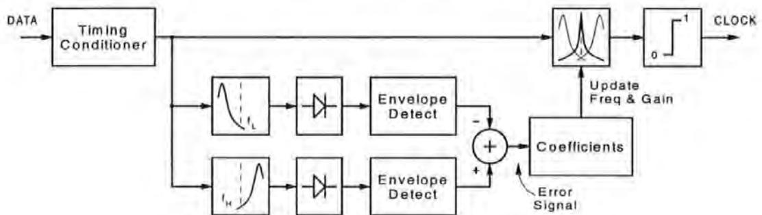
**Figure 3-2 Adaptive clock recovery system**
