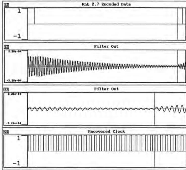
**Figure 2-19 Flywheel performance - RLL2,7 encoded data**
