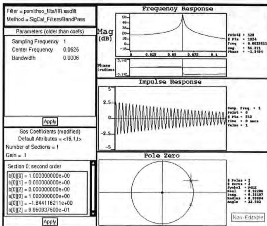
Figure 2-34 IIR Filter quantized to 16 bits
