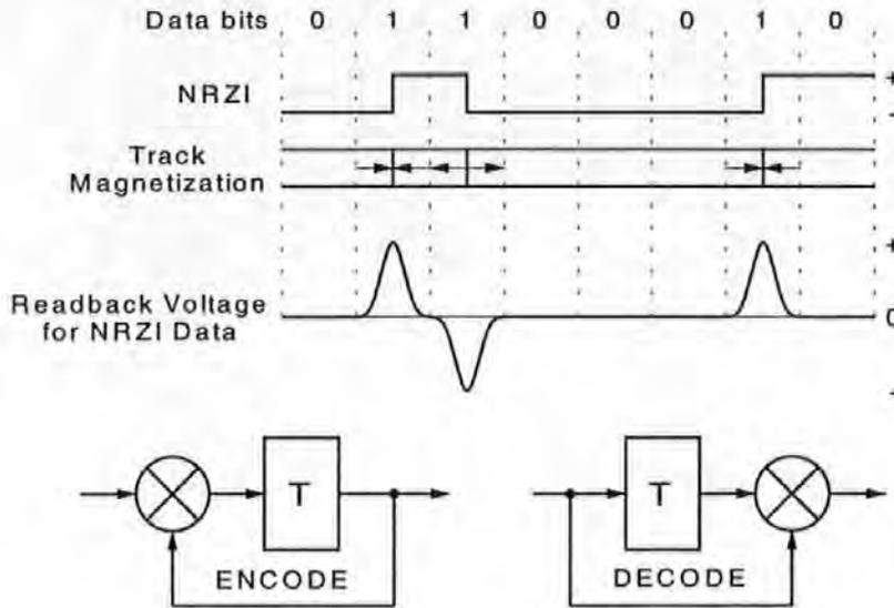
**Figure 1-18 NRZI or differential coding**
