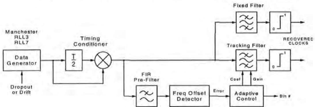
**Figure 3-28 Overview of adaptive simulation model**
