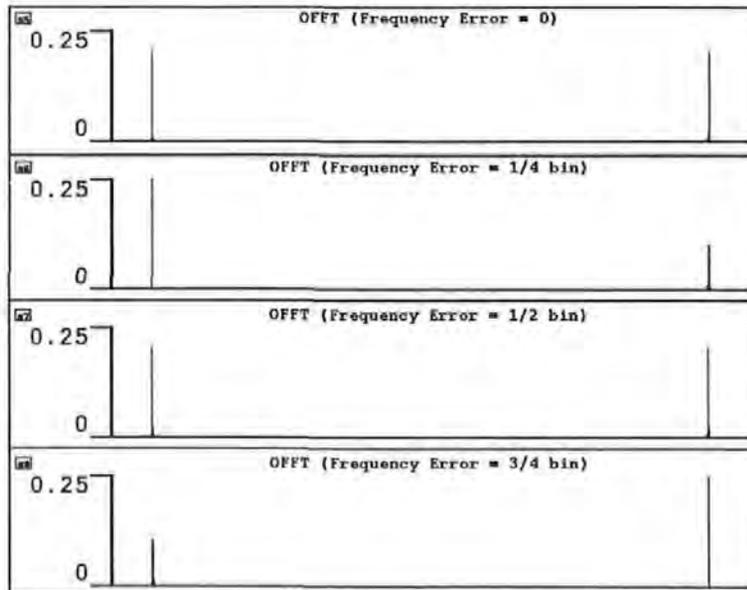
Figure 4-5 Simulation of OFFT with frequency offsets
