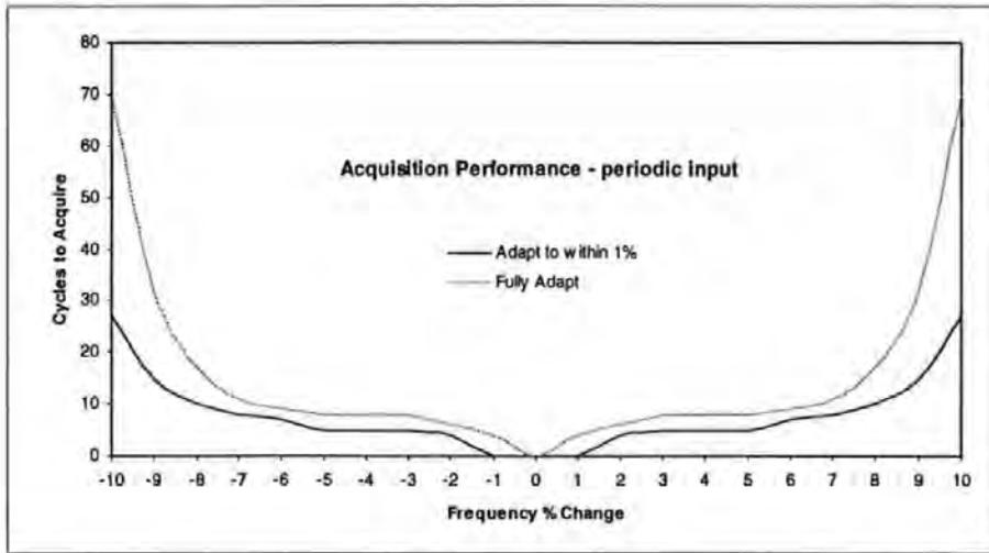
**Figure 3-17 Acquisition performance for a periodic input**
