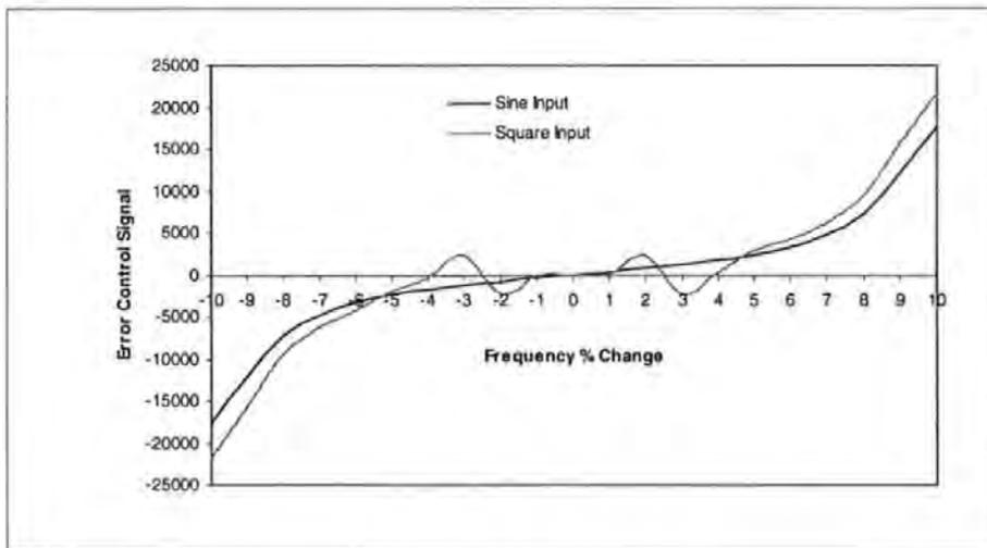
**Figure 3-19 Error control for a signal generator input**
