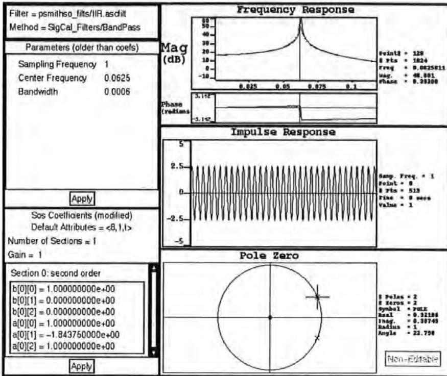
Figure 2-36 IIR Filter quantized to 8 bits
