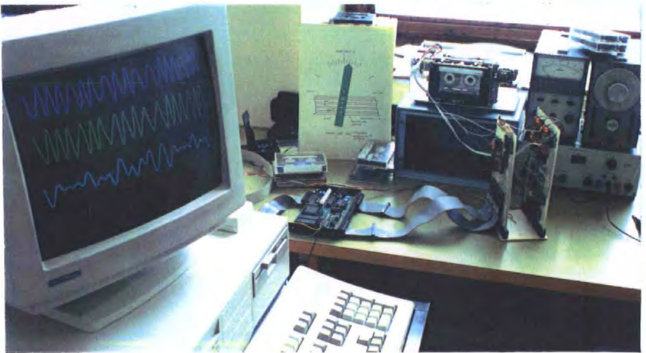
Figure 3.16 Photograph of Recording System employing Sampling Detection
