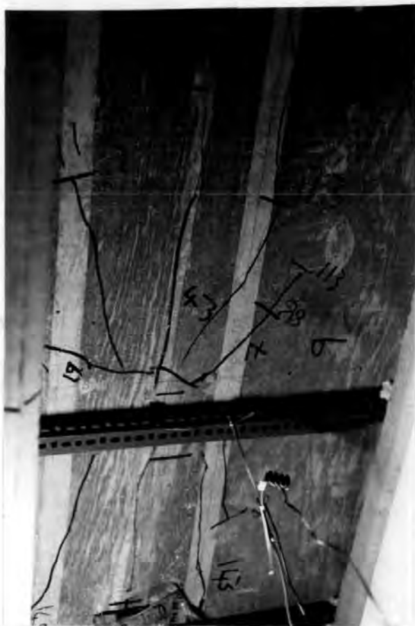
Figure 8.24: Crack pattern under single wheel
