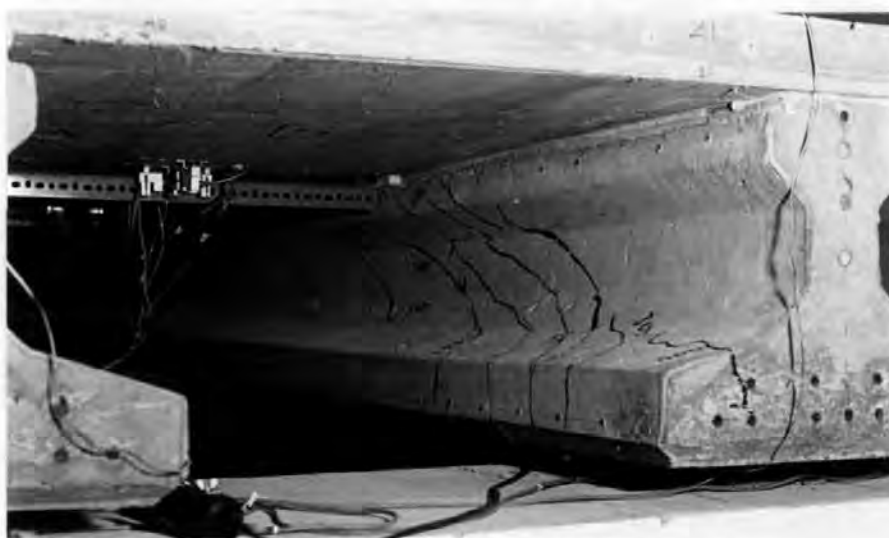
Figure 8.16: Shear cracks in Beam B
