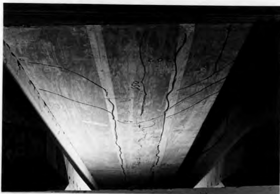
Figure 8.17: Soffit cracks under wheel 4
