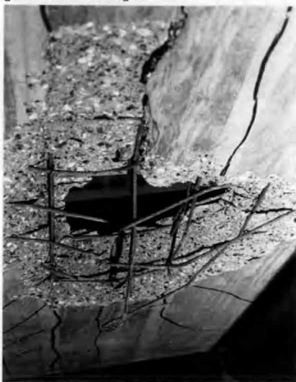
Figure 8.21: Failure cone viewed from below
