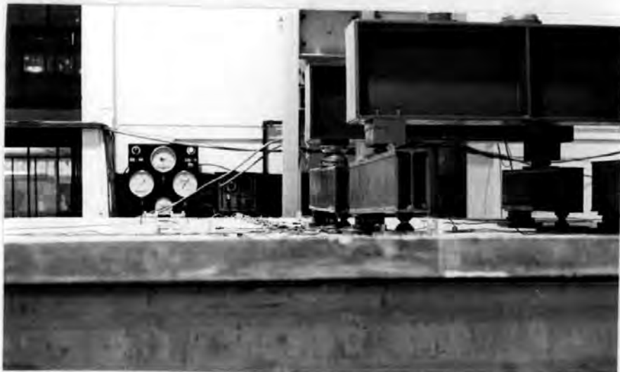
Figure 8.19: View across deck as failure approached
