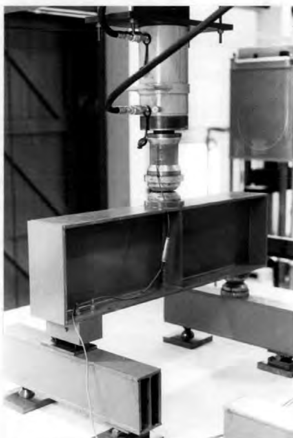
Figure 8.10: Spreader beam assembly
