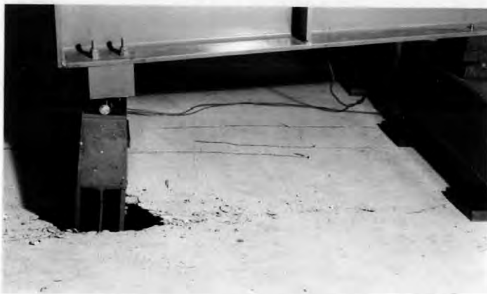
Figure 8.20: Failure; Wheel 4 punched through deck
