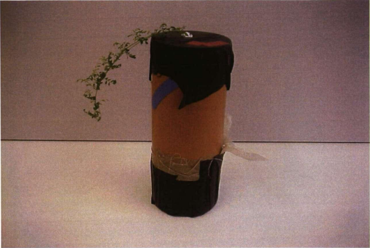
Plate 5.1. To show how the pots were sealed in the lentil experiment.
