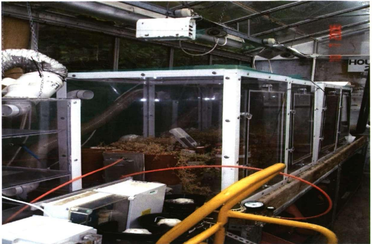
Plate 2.1. The enclosed growth chambers at the end of an experiment. The mixing chamber is on the left of the picture and a Telaire monitors visible in the first chamber.
