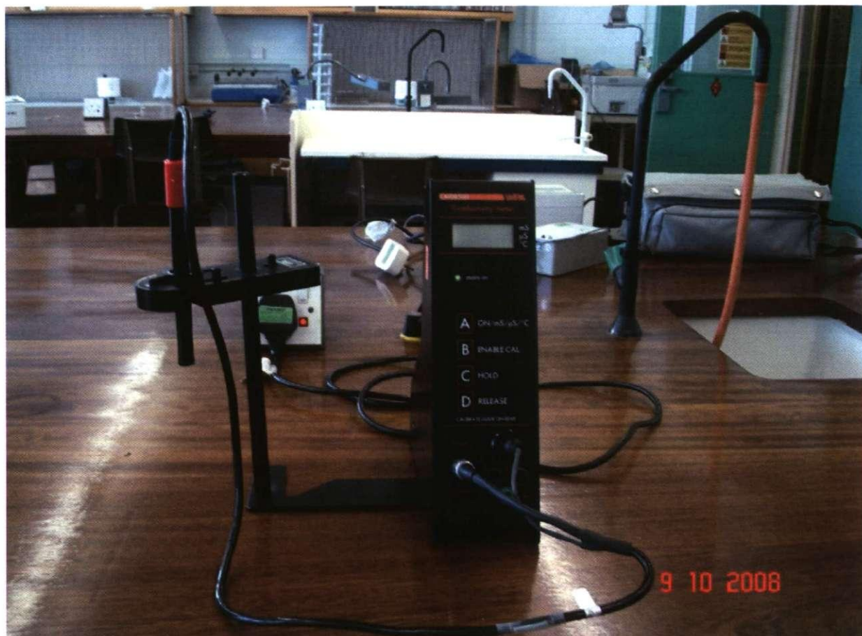
Plate 2.4. Electrical conductivity meter used in the analysis.
