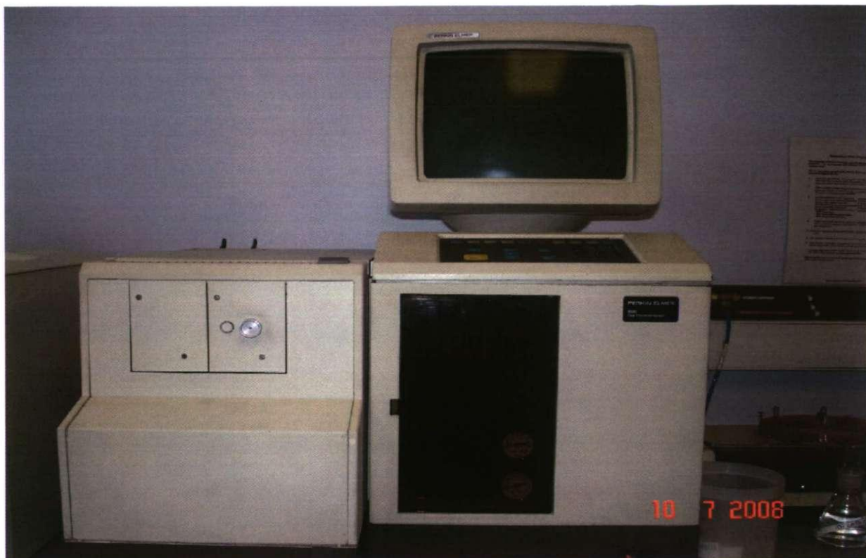
Plate 2.6. Perkin Elmer 8500 gas chromatograph used in the analysis.
