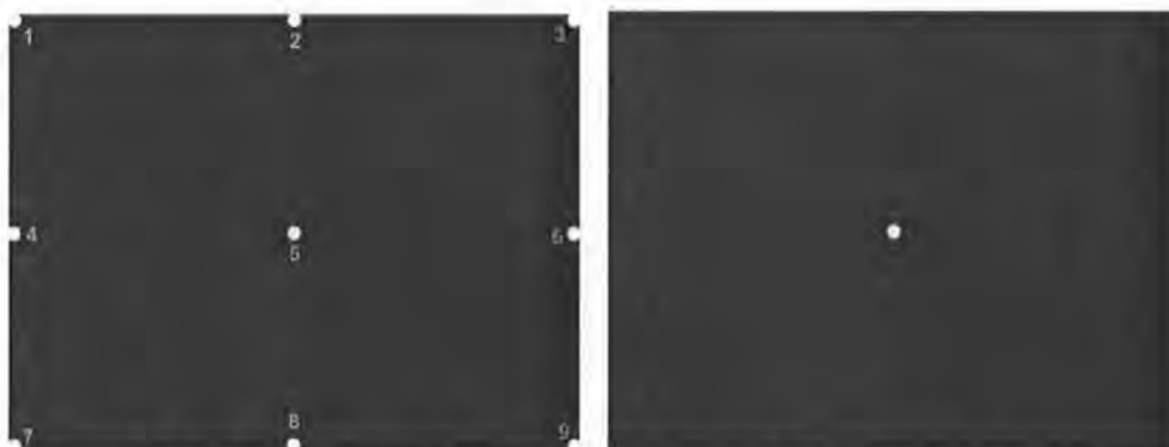
Figure 6.5 The calibration screens used during the trial, (a) 9-point, (b) single point.
