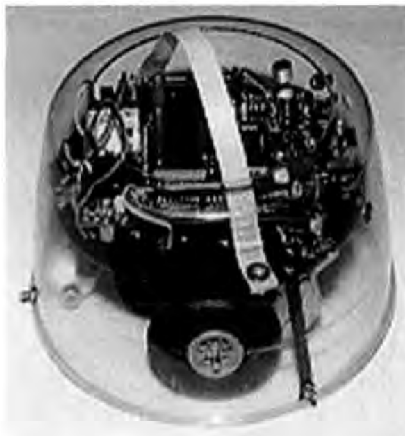
Figure 3.1: The commercial Rug Warrior robot.
