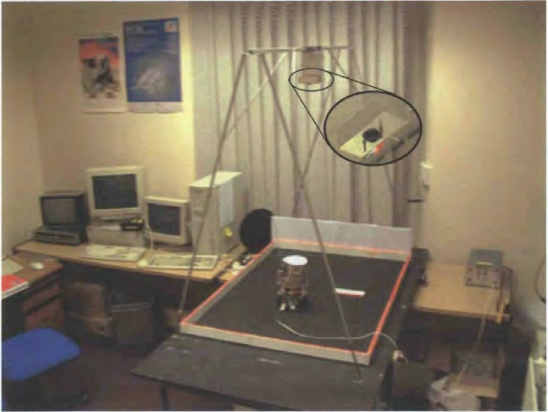
Figure 7.1: The overhead camera setup used to record the robot's motion during the experiments.
