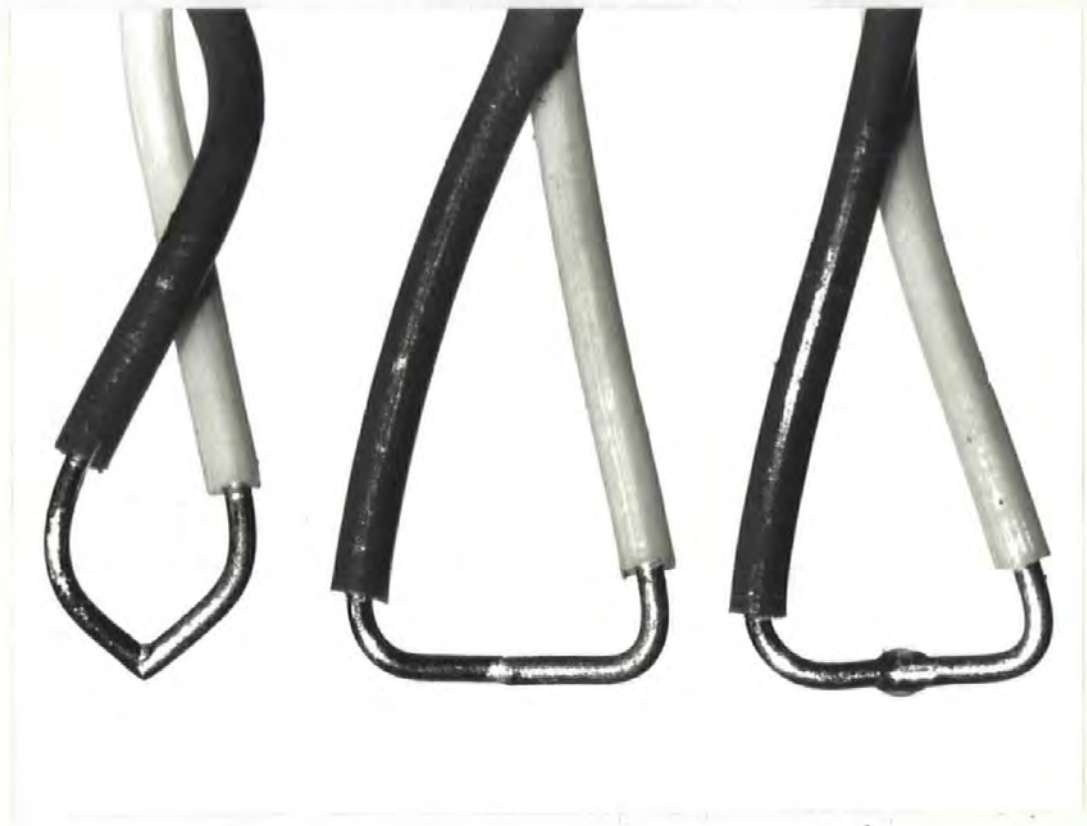
Figure 4. Photograph of the 300 \mu\text{m} diameter thermocouples
