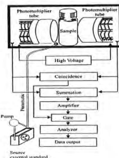
Figure 2.20. Configuration of a typical scintillation counter (Valkovic, 2000).
