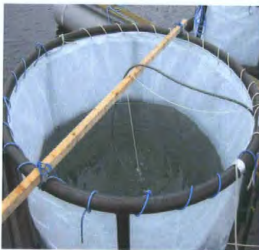
Fig. 2.1. (A) The floating raft with the sea enclosures ( www.ifm.uib.no/batmare/facilities.html ). (B) Detail of one of the enclosures showing airlift system. (Diagram adapted from Egge & Aksnes, (1992)).
