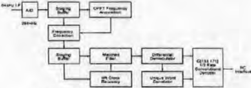
Figure 13 - Burst Demodulator with FEC
