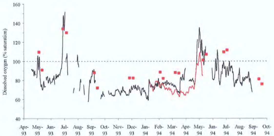
Fig. 4.20. Doodson-filtered dissolved oxygen data from continuous monitoring inside harbour at surface (black line) and bottom (red line) spanning the biologically active seasons of 1993 and 1994. Dashed line denotes 100 % saturation level. Red squares represent routine monitoring results (SH2 surface).
