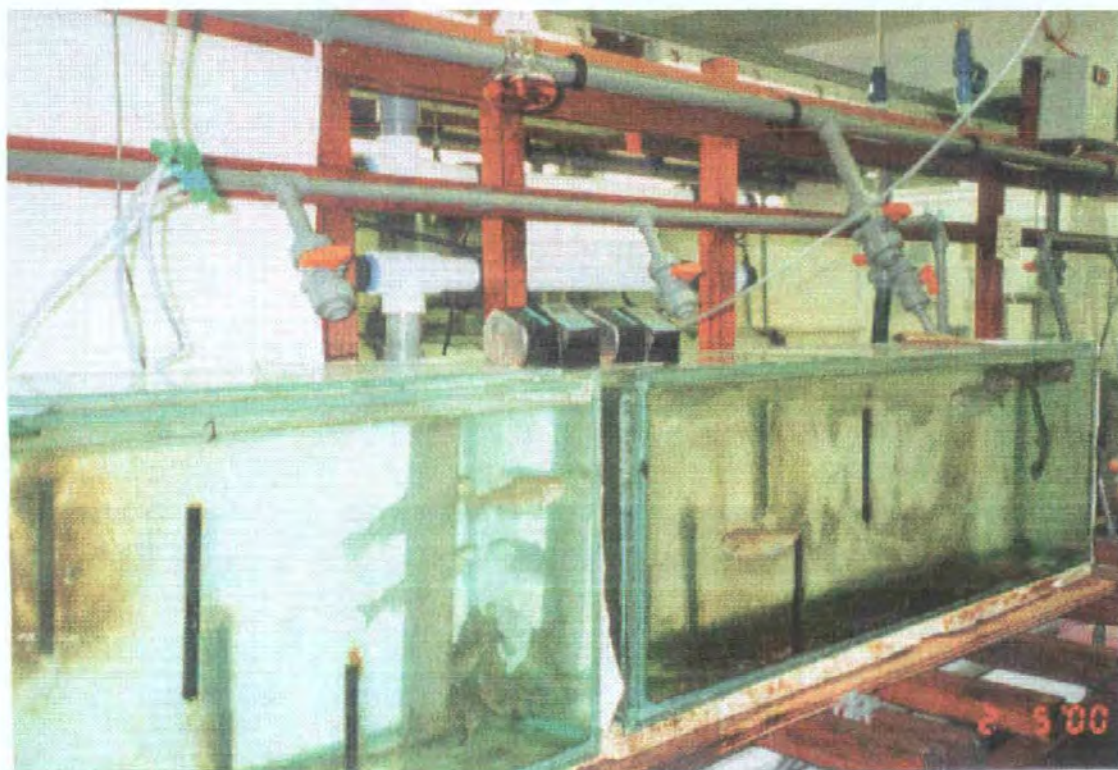
Plate 2. Aquarium system used to monitor effects of Cu-exposure on a point source feeding hierarchy (PS group, n = 10 ). Plate shows automatic feeders (Nutramatic 500) and red light source, used as visual stimulus for food delivery (switched on 1 min prior to feeding). Fish in near tank fed Control diet and far tank a Cu-contaminated diet (730 mg Cu kg -1 feed d.w.). The system above was duplicated, and both systems received water from same biofilter.
