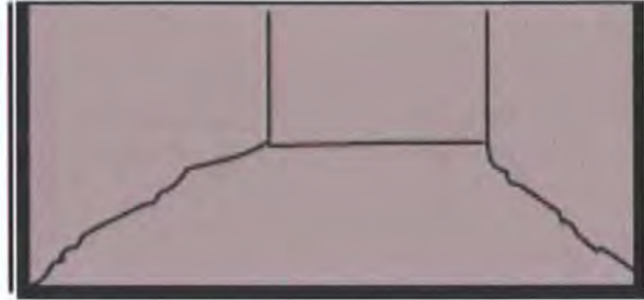
Figure 11 Experimental failure pattern of base panel
