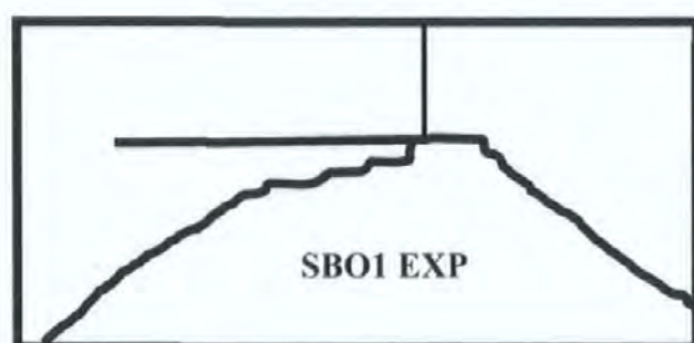
Figure 7.19 the experimental failure pattern of masonry panel SBO1
