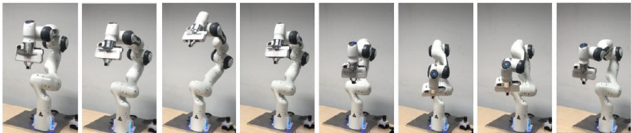
Figure 18. Photo sequence of one periodic movement resulting from the application of the LNN-model-based controller tracking trajectory.
