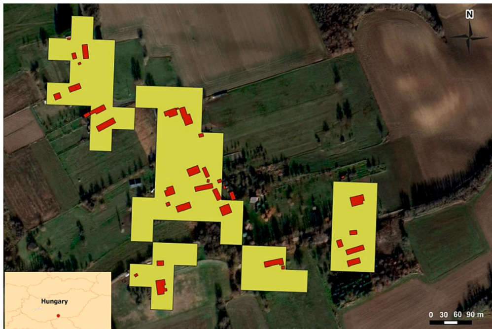
Fig. 3. Comparison of building footprints in the GHSL-based (red polygons) and OSM + MGBF-based (yellow polygons) classifications over a randomly selected rural region of Hungary (bottom left map). (For interpretation of the references to colour in this figure legend, the reader is referred to the web version of this article.)
