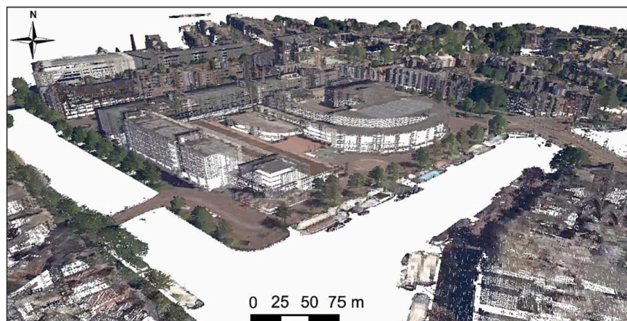
Fig. 5. An example of the LIDAR-based 3D surface models (Rotterdam, the Netherlands) created to estimate roof-specific modelling inputs.
