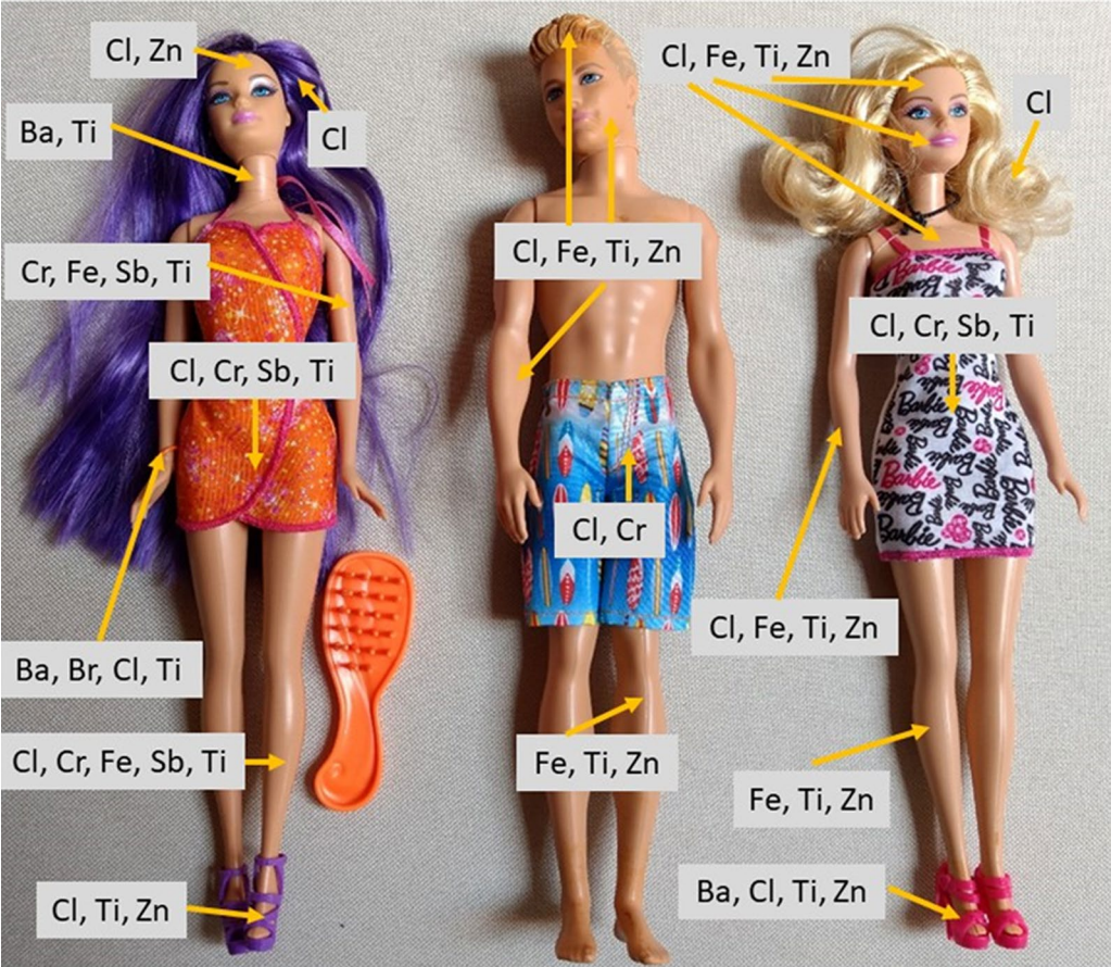
Fig. 1 Elements detected by XRF spectrometry in different components of three Barbie dolls manufactured in 2012. Concentrations determined are given in https://doi.org/10.5281/zenodo.8305228
