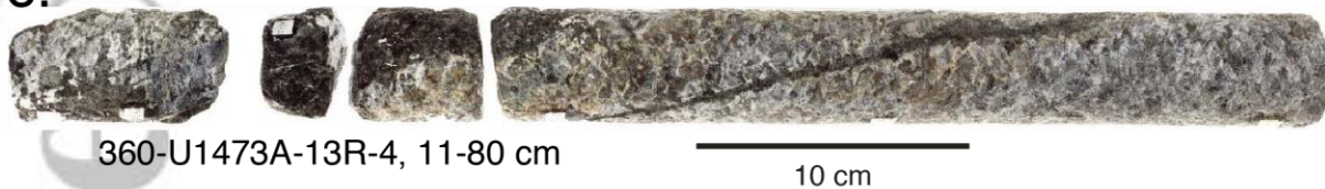
Figure 15. Hole U1473A metamorphic veins: a. Compound amphibole-clinozoisite vein cutting olivine gabbro with alteration corona extending into the fresh olivine gabbro replacing primary Cpx. b. Microphotograph of compound vein in 'A' in plane light consisting of brown and brown-green amphibole sub perpendicular to crystal-plastic foliation, split by a later clinozoisite vein. c. Parallel set of black amphibole veins, one ~5+ mm thick, consisting of mostly of brown and some brown-green amphibole. d. Greenschist facies assemblage in plane light of a felt mass of pale green actinolite and chlorite cutting plagioclase. e. Greenschist facies micro vein crosscutting plagioclase in olivine gabbro consisting of chlorite, zoisite, and actinolite crosscutting plagioclase. f. Yellowish clay microveins crosscutting plagioclase in olivine gabbro. g. Late calcite veins crosscutting a neoblastic domain of plagioclase, Cpx, and olivine in plastically deformed olivine gabbro.
