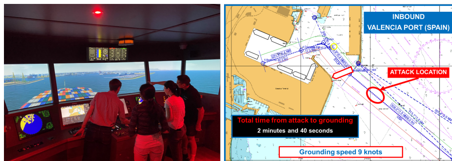
Figure 2: Demonstration of the second scenario jamming of the rudder full to port and engine full ahead inbound to the port of Valencia (Spain). A group of participants in the full bridge ship simulator at the start of the exercise (on the left side) and ECDIS display (with additional information) at the end of the exercise (on the right side)
