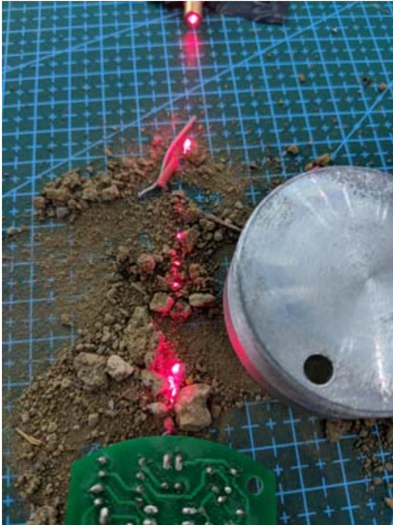
(Fig. 41. Dirt interference with laser light and audio transducer)
