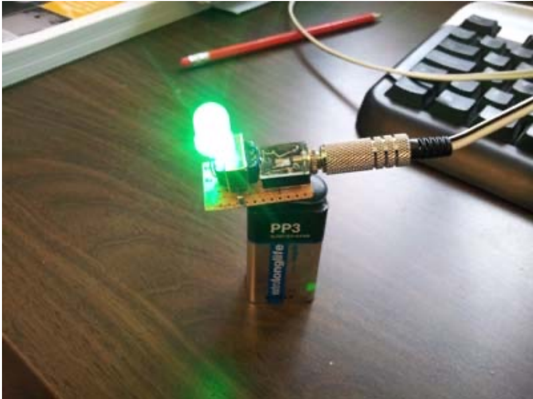
(Fig. 1. LED Transmitter on perforation board)
