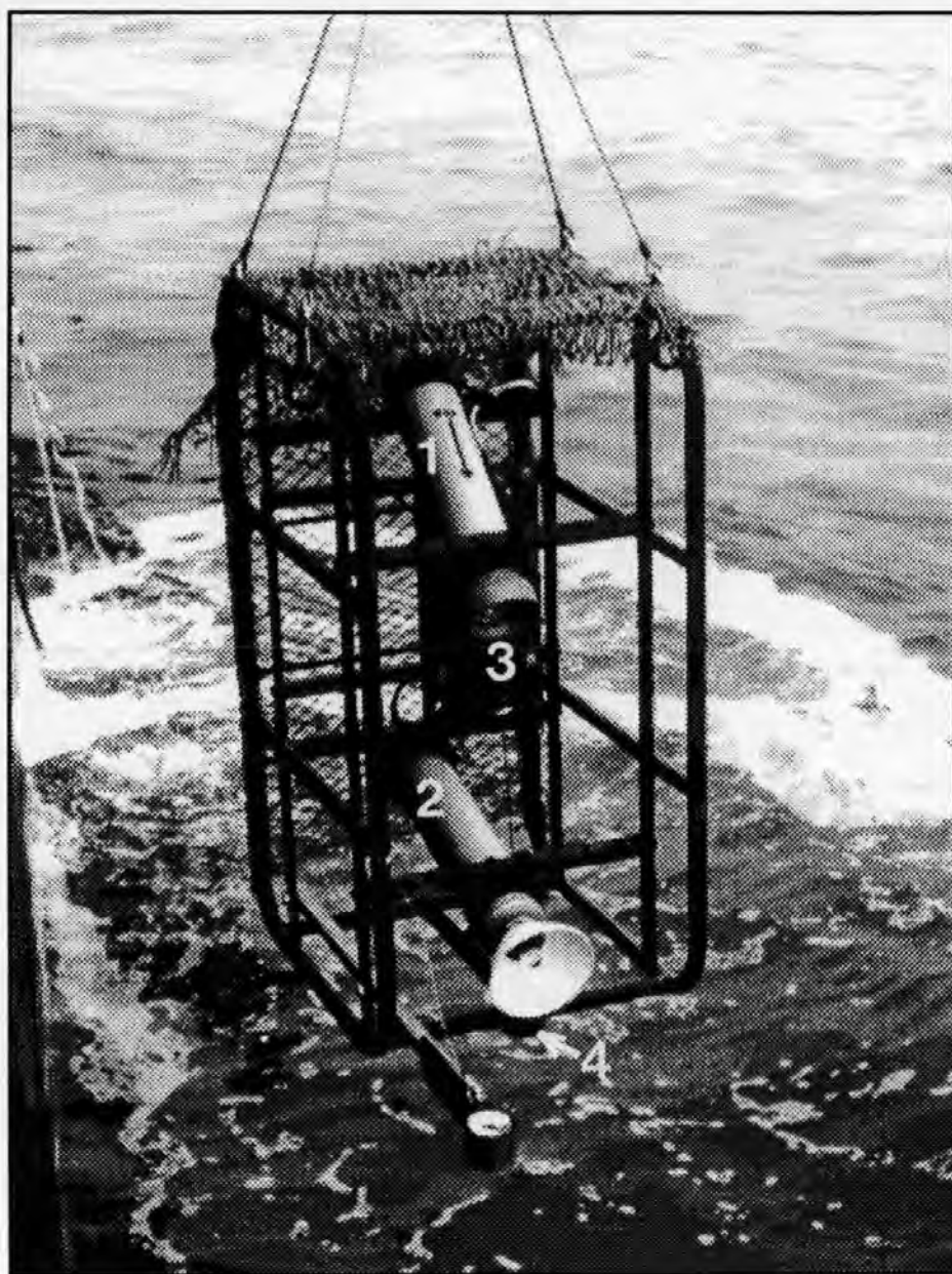
Plate 6.1. "Cage-type" camera assembly used to take seabed photographs at the North Sea study site; (1) camera, (2) flash unit, (3) switch, (4) trigger weight.
