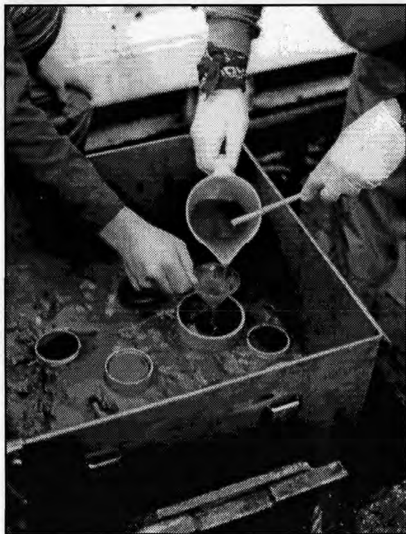
Plate 4.1. Epoxy resin being poured into the burrow openings (enclosed by plastic rings) of Callianassa subterranea aboard R.R.S. Challenger (box core= 0.25m 2 ).
