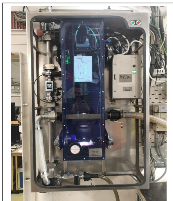
The Plankton Imager, recently developed by Cefas and Plankton Analytics in the UK, is an imaging tool for sampling zooplankton without the need of human intervention. It consists of a high-speed camera that images all passing particles in a flow of pumped seawater. Images are identified in real-time and uploaded via satellite. This system requires no on-board expertise, harmful chemicals, or deployment of gear from the ship. It can collect data at a significantly finer spatial resolution than traditional methods. It also measures zooplankton, supporting carbon accounting. In its current state of development, its main capability is counting copepods.
