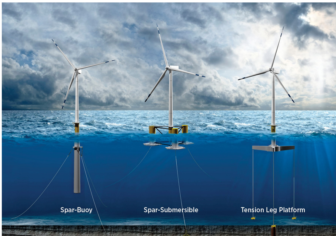
Figure 1.5: Types of floating offshore wind turbines (Source: IRENA (2016b) ) (Permission has been granted by IRENA/Joshua Bauer of NREL to reproduce this figure)
