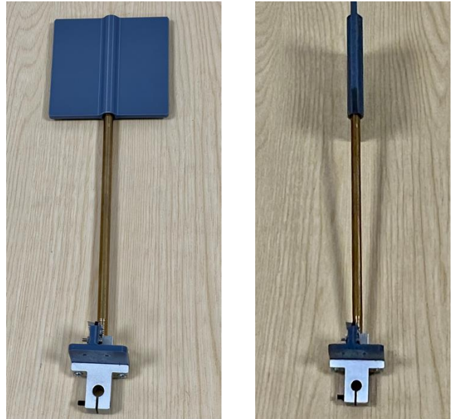
Figure 5: The pendulum paddle can be rotated, thus adjusting the viscous drag due to air resistance from low to high values.
