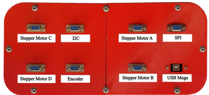
Figure 23. View of the actual controller panel cover, which was designed in Autodesk Fusion 360 and then 3D printed.
