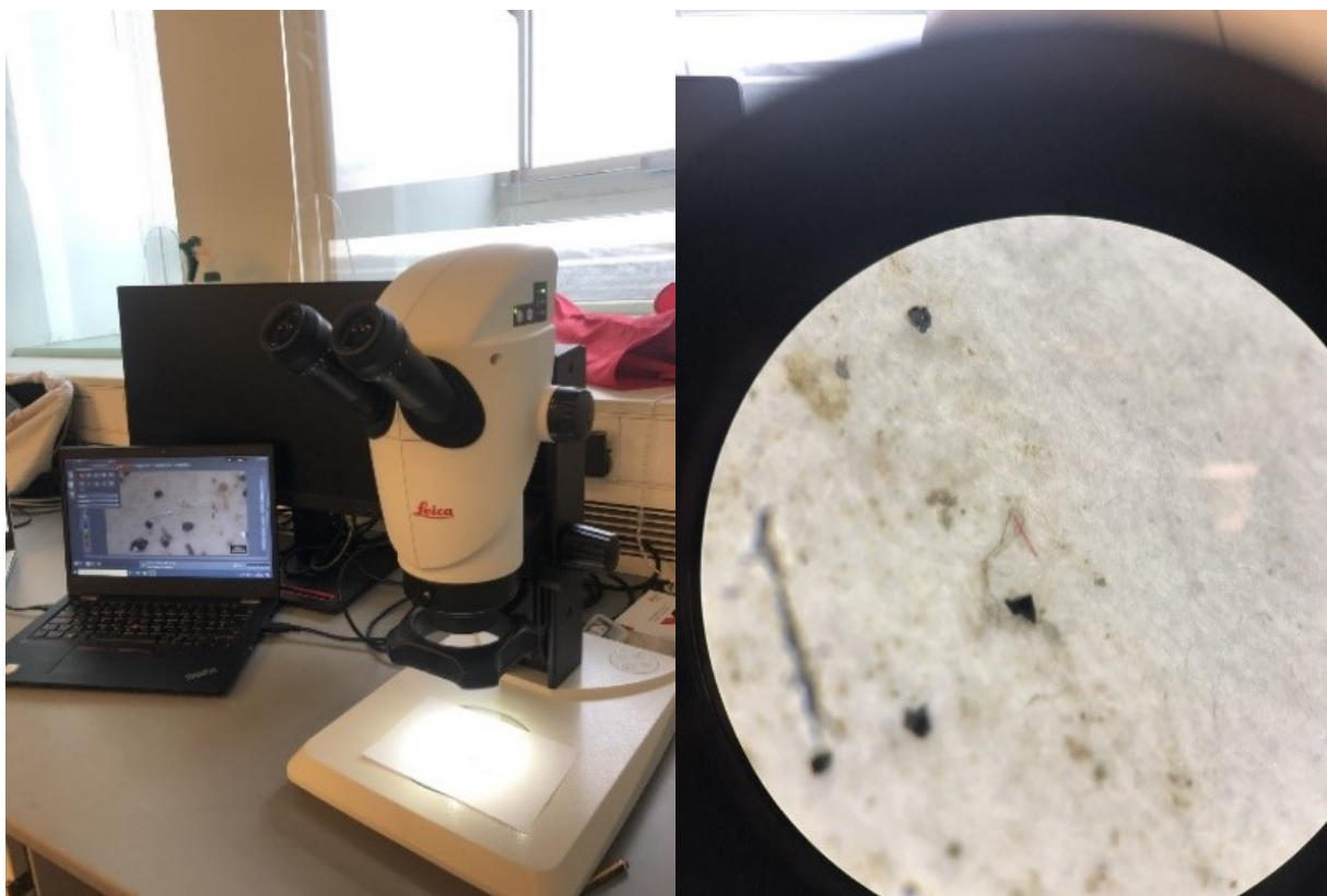
Figure 5: Images of the microplastic analysis setup. On the left is the stereomicroscope with a camera attachment showing one of the paper filters. On the right is a closer image showing what could be seen through the microscope.
