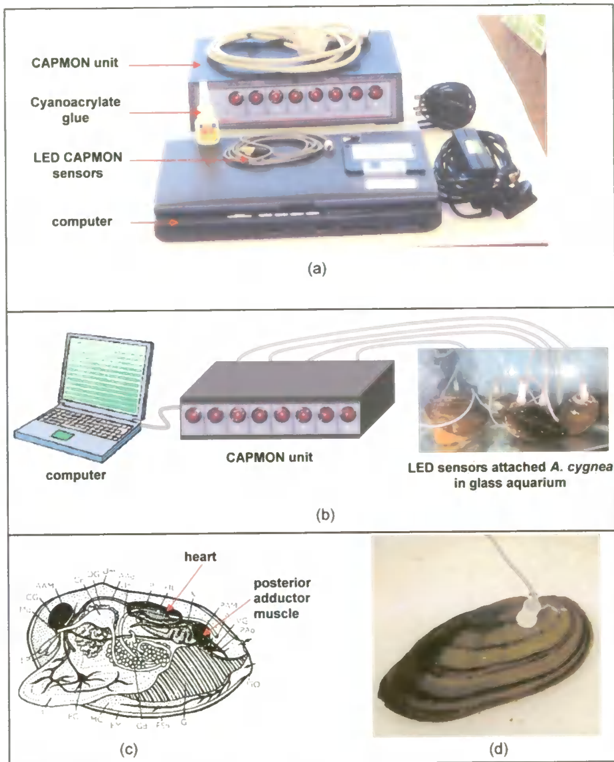
Figure 6.3: (a) Apparatus needed for monitoring cardiac activity using the CAPMON; (b) set-up of CAPMON to monitor cardiac activity of A. cygnea ; (c) schematic diagram of location of the mussel heart (source: Janus, 1965); (d) CAPMON LED sensor attached to A. cygnea , placed over heart
