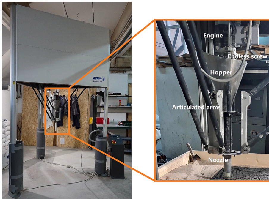
Fig. 9. 3D printer system details.
