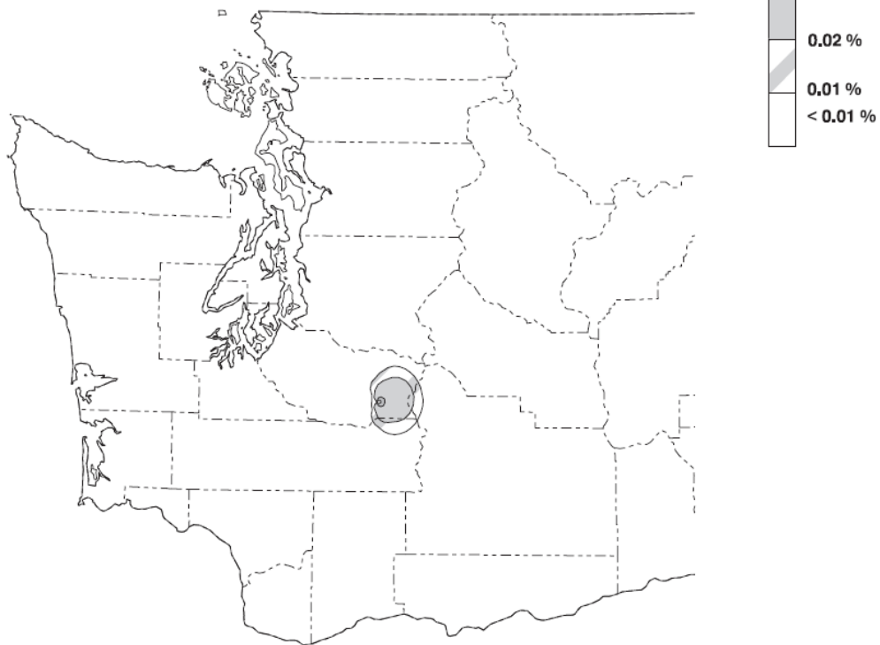
(2) Annual probability of the deposition of 10cm or more of tephra from Mount Rainier.
